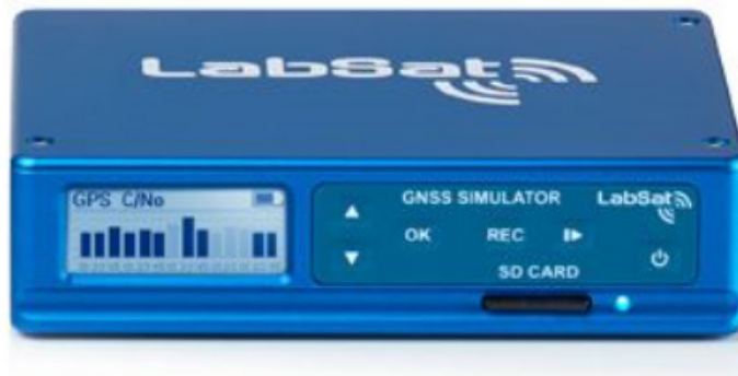
Figure 34. LabSat GNSS simulator. Source: Racelogic Ltd (2019).
