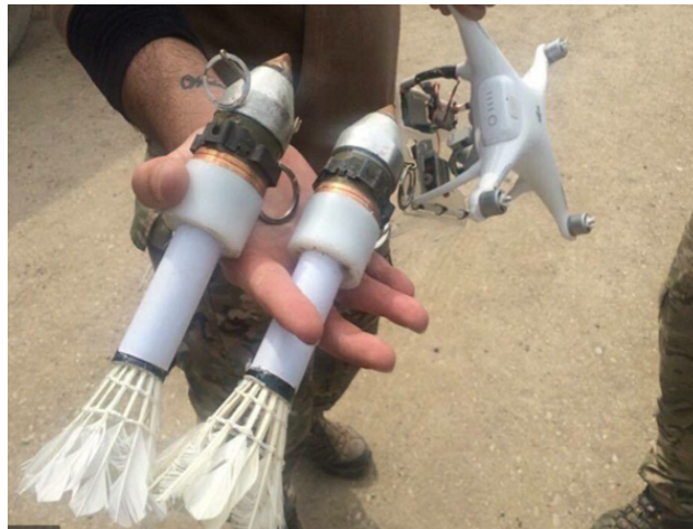
Figure 13. A COTS drone rigged with an explosive payload. Source: Pomerleau (2017).
