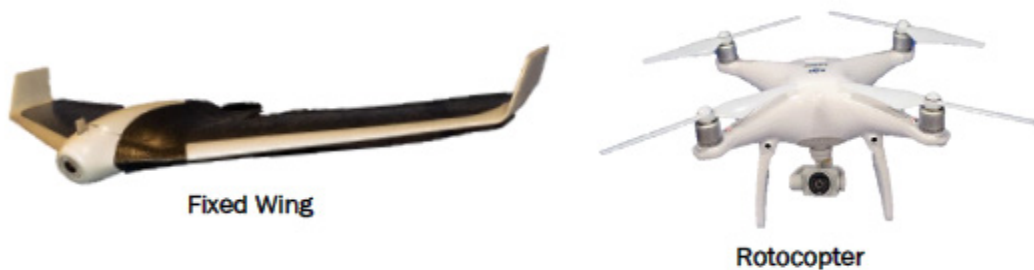
Figure 4. Fixed-wing and rotocopter design UAV. Source: DHS (2019).
