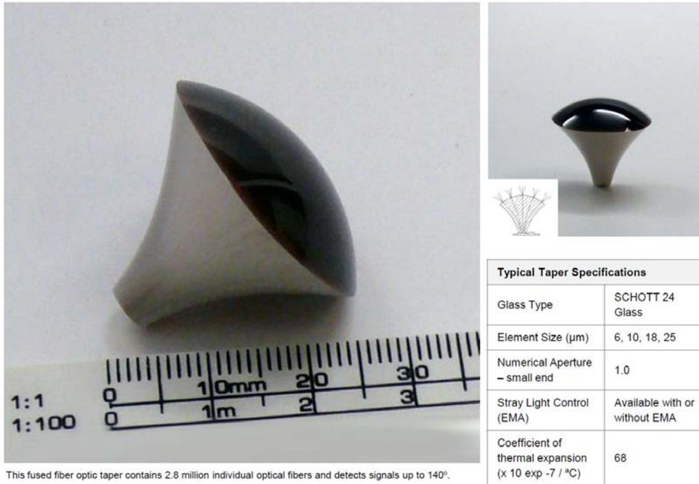
Figure 30. SCHOTT Dragonfly Directional Sensor. Source: Geary et al. (2013)
