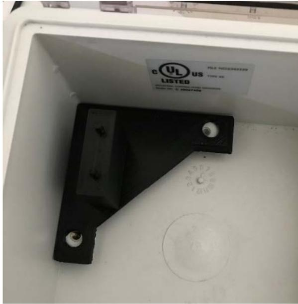
Figure 26. 3D Printed Platform for Arced Phototransistor Array
