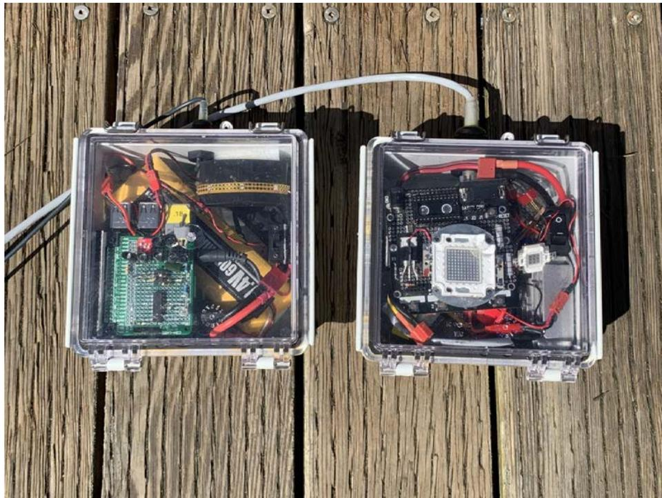
Figure 34. Receiver (left) and Transmitter (right) Prototype
