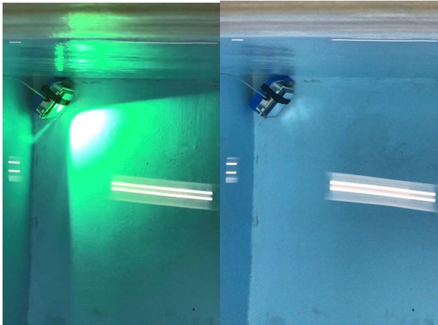
Figure 29. VLC Transmitter Operating in Clear Water
