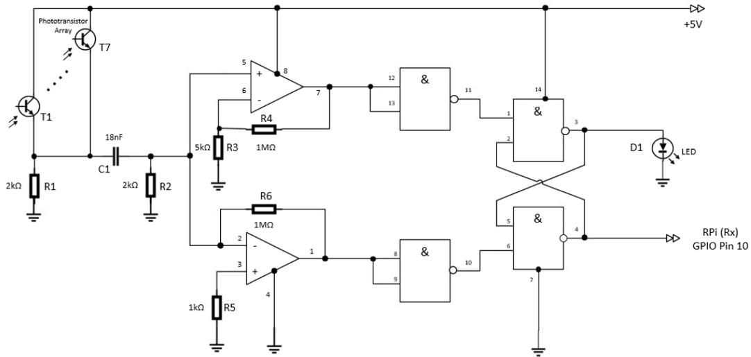
Figure 22. Phototransistor Array Receiver Prototype Schematic
