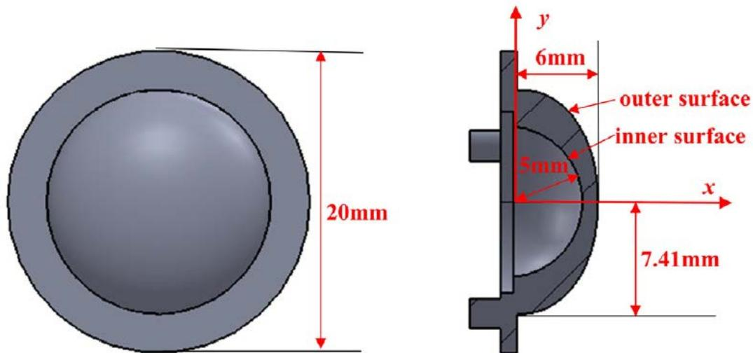
Figure 12. Quasi-omnidirectional Transmitter. Source: Han et al. (2018).
