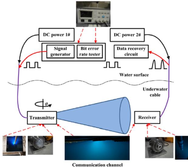
Figure 15. Experiment Design with Transmitter and Receiver Submerged.
