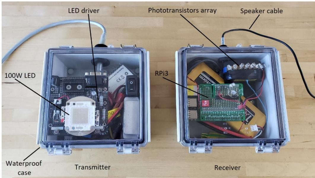
Figure 28. Waterproofed VLC Transmitter and Receiver Systems
