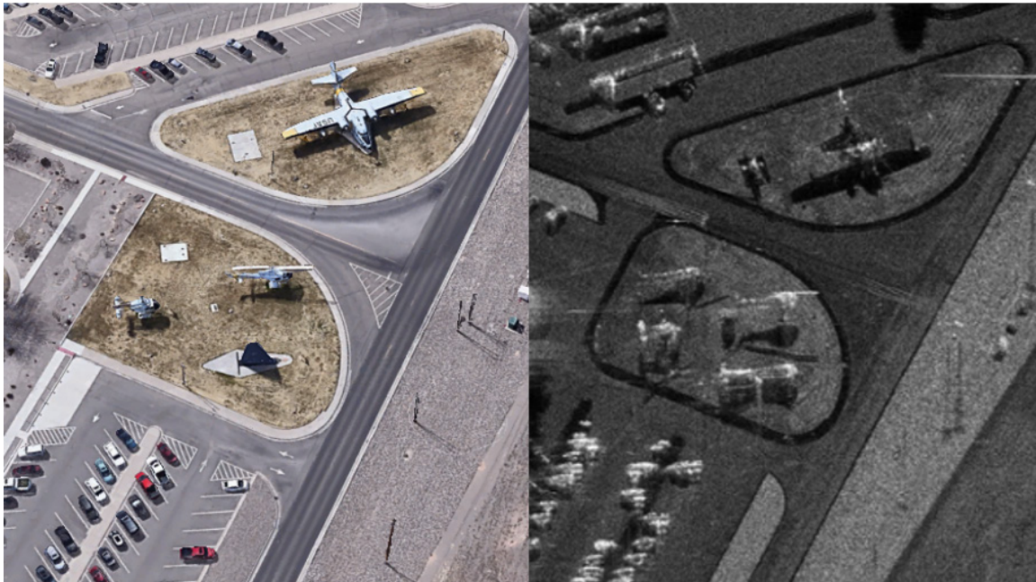
Figure 1. Comparison of EO and SAR Overhead Images. Adapted from Google (n.d.) and Sandia National Laboratories (n.d.).
