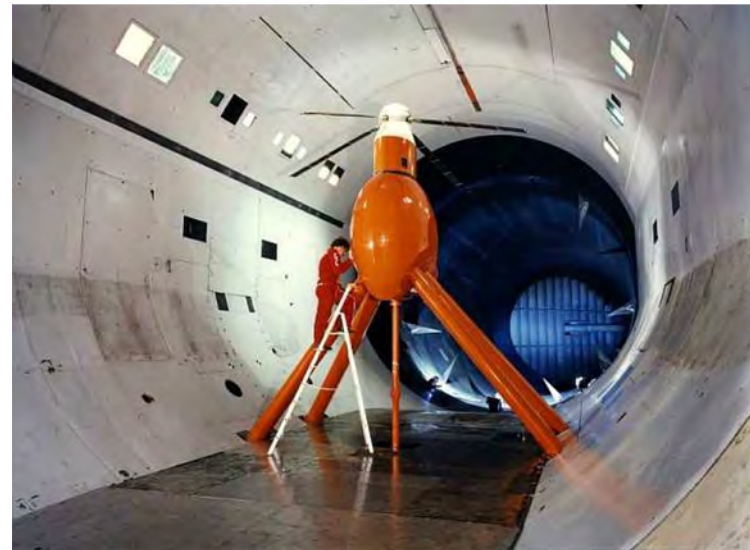
7A ROTOR ONERA S1MA WIND TUNNEL MODANE, FRANCE 1991
