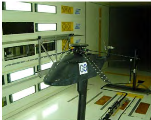
GOAHEAD in DNW-LLF wind tunnel
