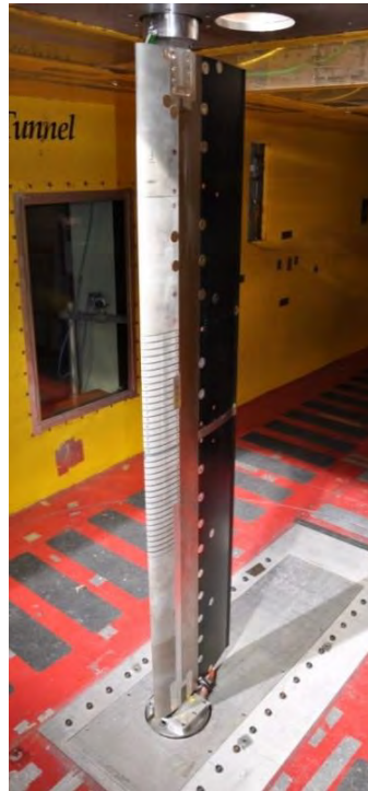
VR-12 model in NASA Glenn IRT
