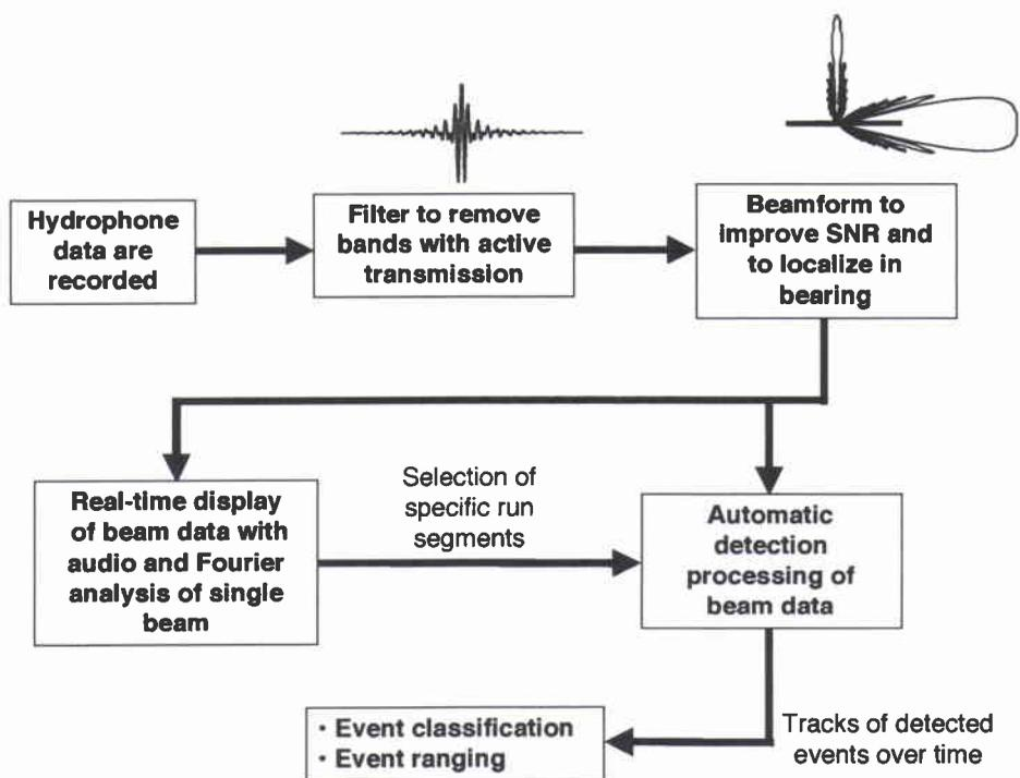
Figure 1 *Flow diagram of signal processing.*
