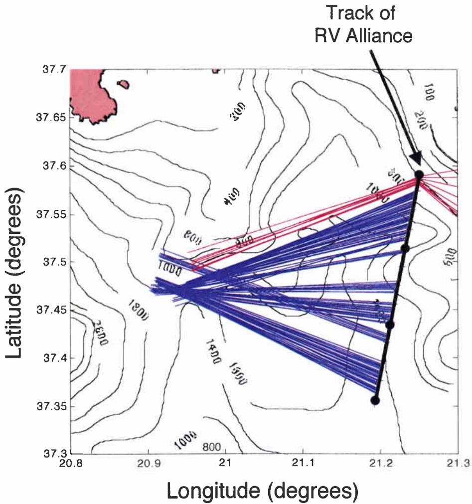
**Figure 14** Lines along bearings of detections for events 2, 3, 5, 6, 8, 12, 13 and 17 of Run 9. Each line is 15 nautical miles in length. Red lines are from event 2 and illustrate localization of a sperm whale to west side of the track of RV Alliance.
