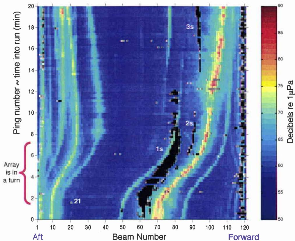
**Figure 11** ENR of detected events from first 20 minutes of Run 9 (gray scale) overlaid on background noise and interference power (color scale).
