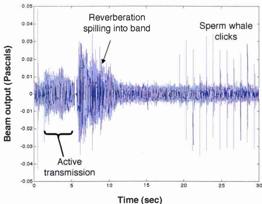
**Figure 5** Example of filtered and beamformed data with sperm whale click train.
