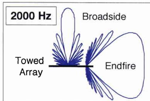
Figure 4 *Beampatterns for MF array.*
