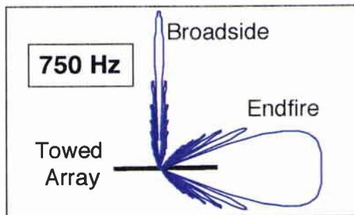
Figure 3 Beampatterns for LF array.
