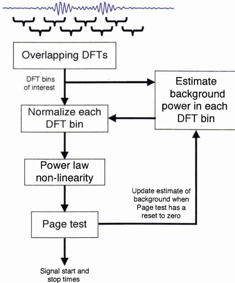
Figure 9 Block diagram of detection scheme.
