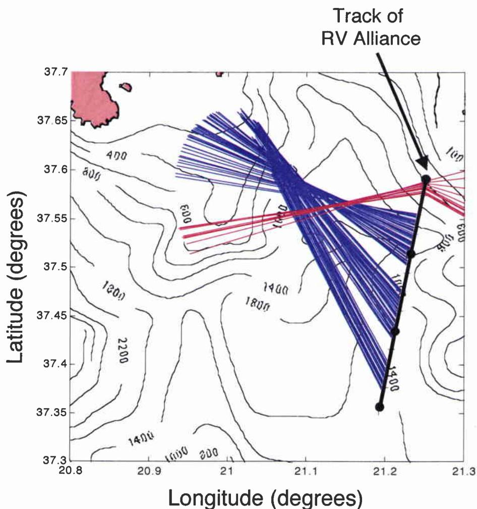
**Figure 13** Lines along bearings of detections for events 1, 4, 10 and 15 of Run 9. Each line is 15 nautical miles in length. Red lines are from event 1 and illustrate localization of a sperm whale to west side of the track of RV Alliance.
