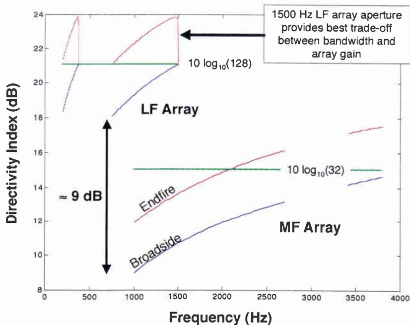
**Figure 2** *Directivity index vs. frequency for different array apertures.*
