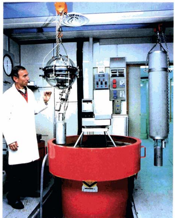
Density bath for depth setting of ocean current drift floats.
