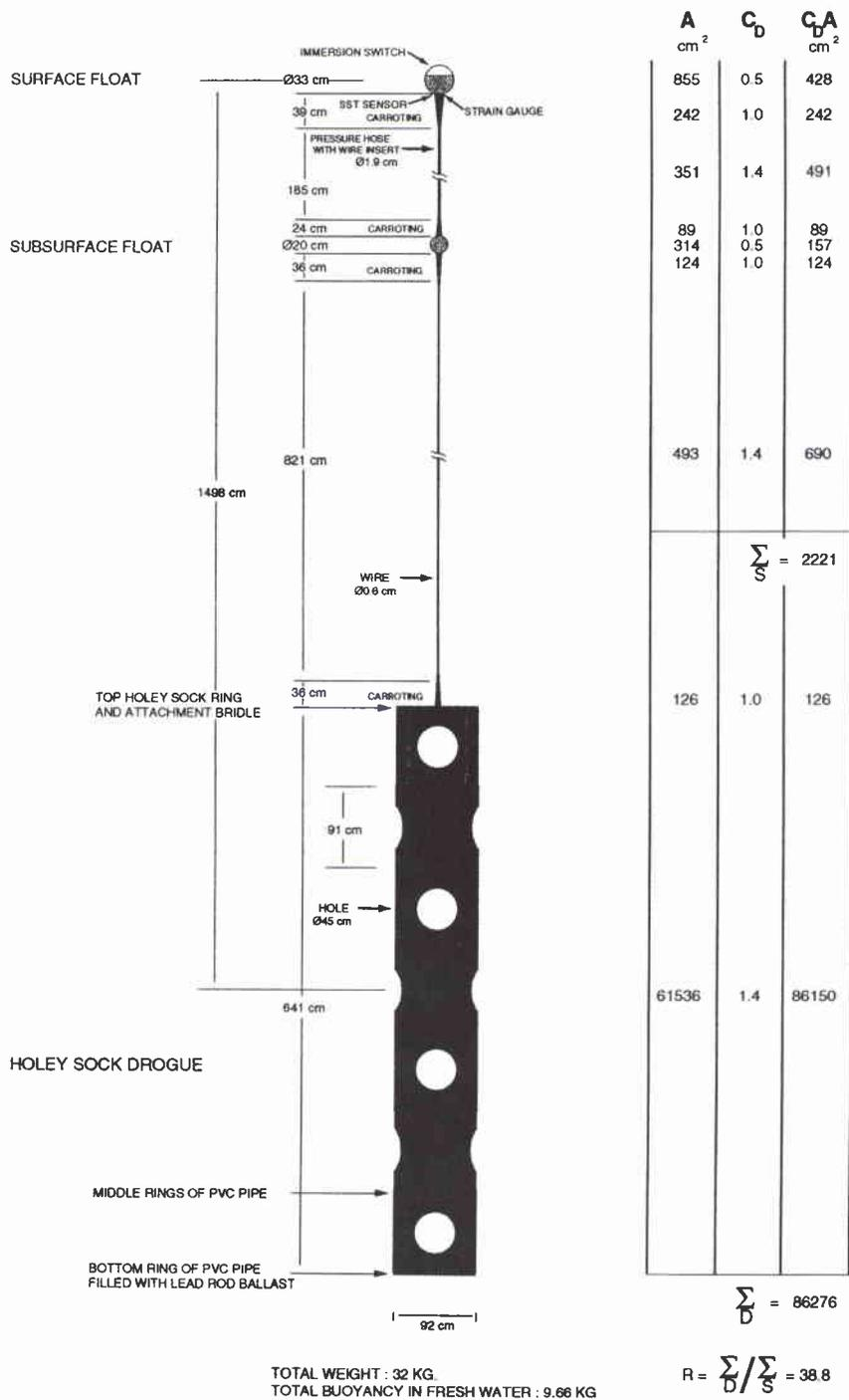
**Figure 1** Schematic diagram of the WOCE/TOGA Lagrangian drifter with computation of drag area ratio (a). Photograph of a WOCE/TOGA drifter recovered after 8 months in the Norwegian coastal current: (b) Global view with Holey sock drogue in the foreground; (c) Detailed view of the surface and sub-surface spheres. The SST sensor is apparent on the surface float.
