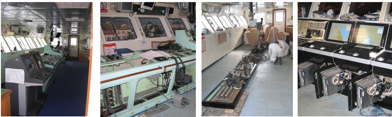
Alliance's makeover, from left: Bridge before the new IBNS (Integrated Bridge Navigation System) was installed, removal of old bridge system, preparing for the new units, new units in the process of installation.
