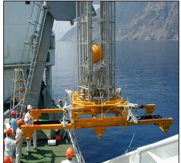
Engineering staff deploying a multi-sensor tower during a sea trial.
