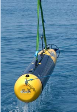
AUV being tested for automatic target recognition and sensor-based navigation
