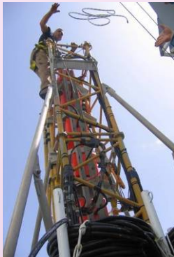
Engineering staff getting ready to deploy the topas acoustic source tower at the FAF 06 sea trial
