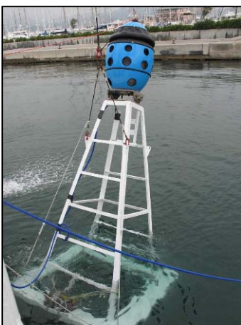
QinetiQ's Cerberus sonar being deployed to the harbour seafloor on a 5m tower
