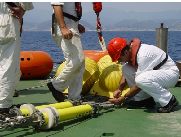
Preparation for the deployment of the EARs (Environmental Acoustic Recording System) buoy which were to be positioned at 1000 m depth for continuous sound recording during Sirena06
