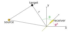
Fig. 1 A bi-static source–target–receiver example, where x and y are the coordinate system, r is the range between target and receiver, and  $\theta$  is the bearing between the array heading  $\phi^R$  (as measured counterclockwise from the x axis) and the target
