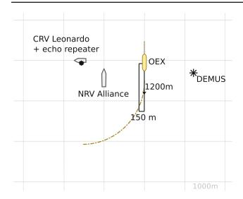
Fig. 9 Static target scenario with anticipated AUV movement. The OEX starts in a southbound racetrack, the 'target' (CRV Leonardo+echo repeater) is static, as are the NRV Alliance and the DEMUS source. Grid size 1.000 m
