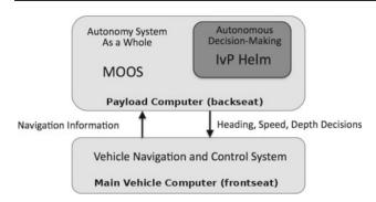
Fig. 5 The frontseat-backseat paradigm as used in MOOS-IvP. The key idea is the separation of vehicle autonomy from vehicle control [8]
