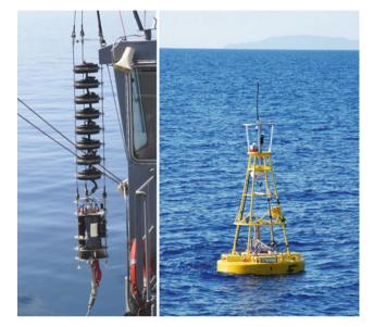
**Fig. 3** Left the DEMUS source during deployment; the eight free-floode ring transducers are clearly visible. Underneath the rings are the electronics. *Right* the DEMUS radio buoy
