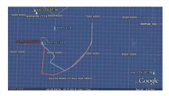
Fig. 11 Command and control centre (alliance) display, third demonstration static target; the AUV (oex\_harpo/e-oex\_2) is optimizing for a static target (leonardo), using on-board active sonar processing (source: demus\_source). The AUV's position updates are received via two acoustic modems, indicated by e-oex\_2 (light blue) and oex\_harpo (red). trk\_\*'s are tracks sent from the AUV via acoustic communications to the command and control centre display. Grid size 100 m
