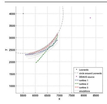
Fig. 12 Overlay of fiel demonstrations on simulation results for the static target scenario. Inter-simulation differences are due to differences in start time of the data stimulator
