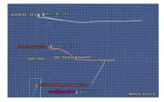
Fig. 13 Command and control centre (alliance) display, firs demonstration moving target; the AUV (oex\_harpo/e-oex\_2) is optimizing for a moving target (leonardo), using on-board active sonar processing (source: demus\_source). The AUV's position updates are received via two acoustic modems, indicated by e-oex\_2 (light blue) and oex harpo (red). ttm \* indications are radar tracks
