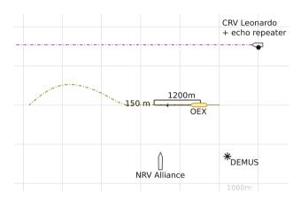
**Fig. 10** Dynamic target scenario with anticipated AUV and 'target' movement. The OEX starts in a westbound racetrack, the 'target' (CRV Leonardo+echo repeater) starts to the northeast in a westbound movement. The NRV Alliance and DEMUS source are static. Grid size 1,000 m
