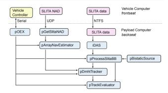
Fig. 6 The OEX's active sonar on-board processing chain
