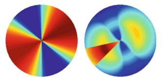
**Fig. 8** Individual BHV\_MinLocErr (*left*) and collective (*right*) objective functions plots from IvP, taken while the AUV is optimizing. *Red* (around 65 and 235 degrees in the individual plot, and the slice around 240 degrees in the collective plot) equals high preference and *blue* (around 155 and 335 degrees in individual and outer boundaries of collective plot) equals low preference. Speed is displayed along the radius, heading in 360°, depth is not shown
