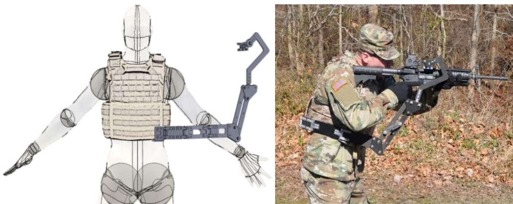
**Fig. 1** CCDC Army Research Laboratory's Third Arm exoskeleton prototype
