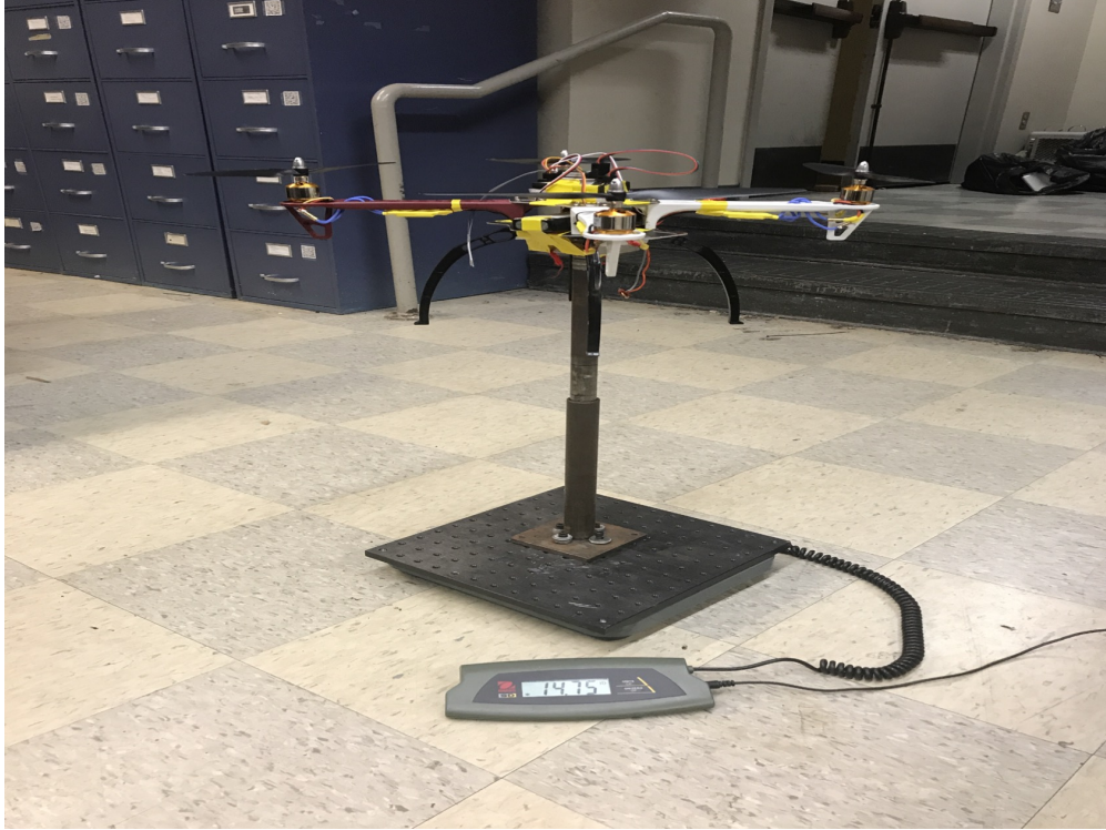
Figure 7: Single quad rotor from the scalable UAV shown during indoor load calibration
