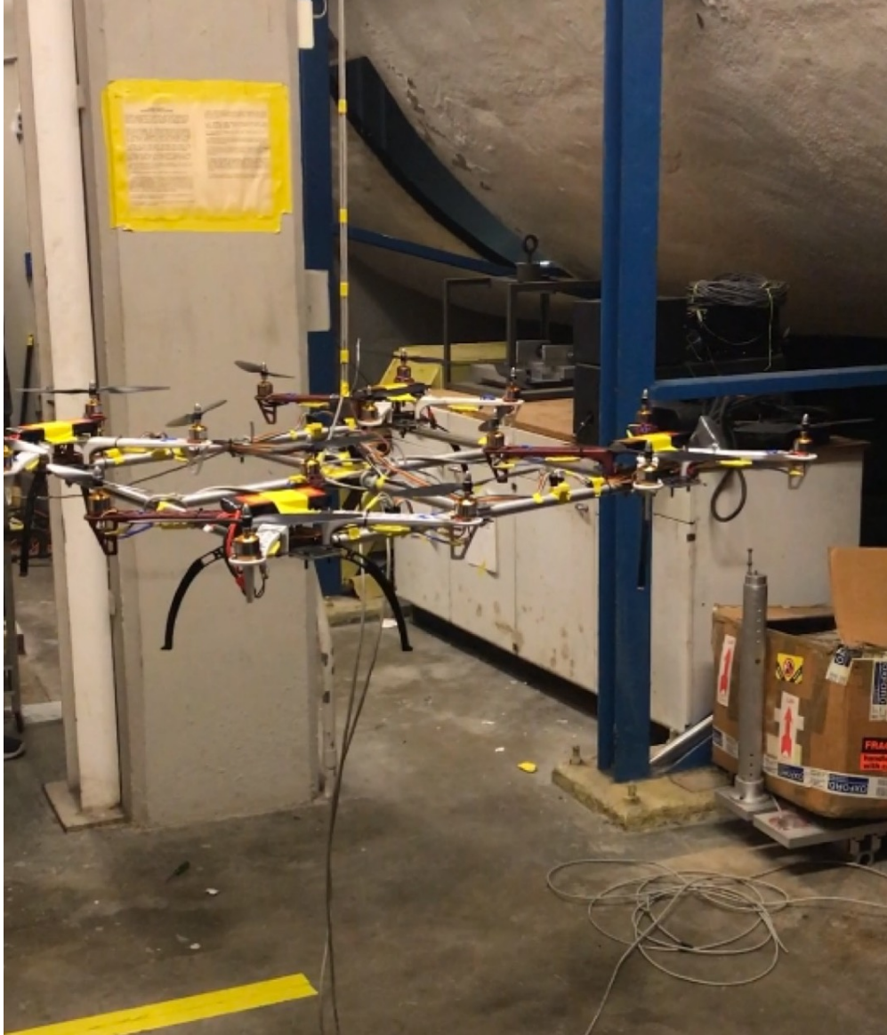
Figure 6: Quad-quad rotor scalable UAV shown during indoor testing
