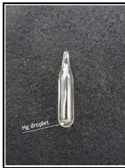
Figure 3: Hg lamp from a Hg + clock supplied to Aerospace by JPL.
