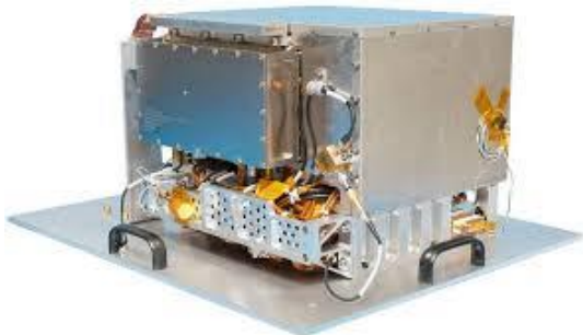
Figure 1: The DSAC Hg + atomic clock [6].
