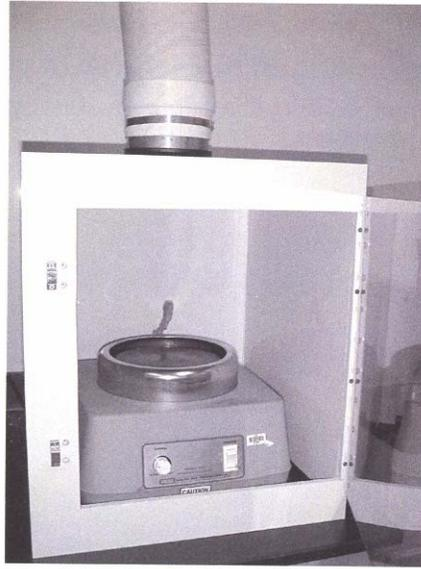
Figure 4. Model 900™ Grinder/Polisher from South Bay Technology.
