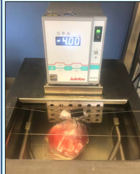
VCA supercooling. Swine partial hind limb stored in a sterile bag in HTK. Chiller set at -4C.
