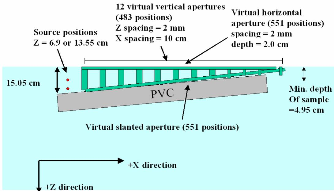
Figure 2 – Experimental setup for runs with the slanted PVC sheet. The dimensions of the sheet are the same as in Figure 1. The slant angle of the sheet is between 4.7 and 4.8 degrees relative to horizontal. The virtual horizontal and slanted apertures consist of 551 records (receiver positions) each. See Table 3 for the relevant data files and plots.
