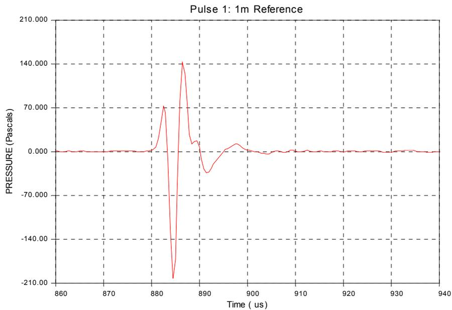
Figure 3 - Temporal response of the source/receiver separated by 1 m.
