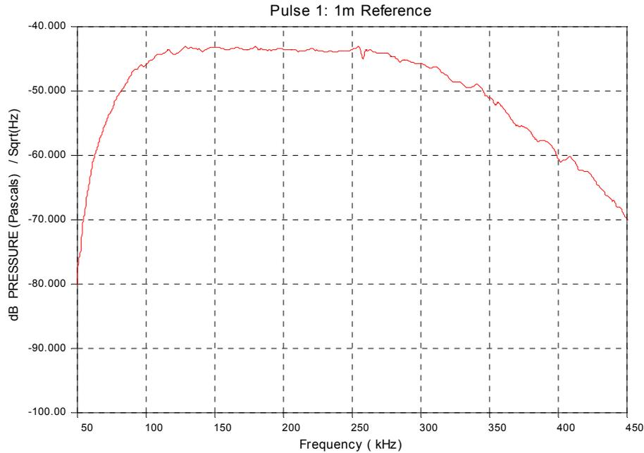
Figure 4 - Frequency response of the source/receiver separated by 1 m.
