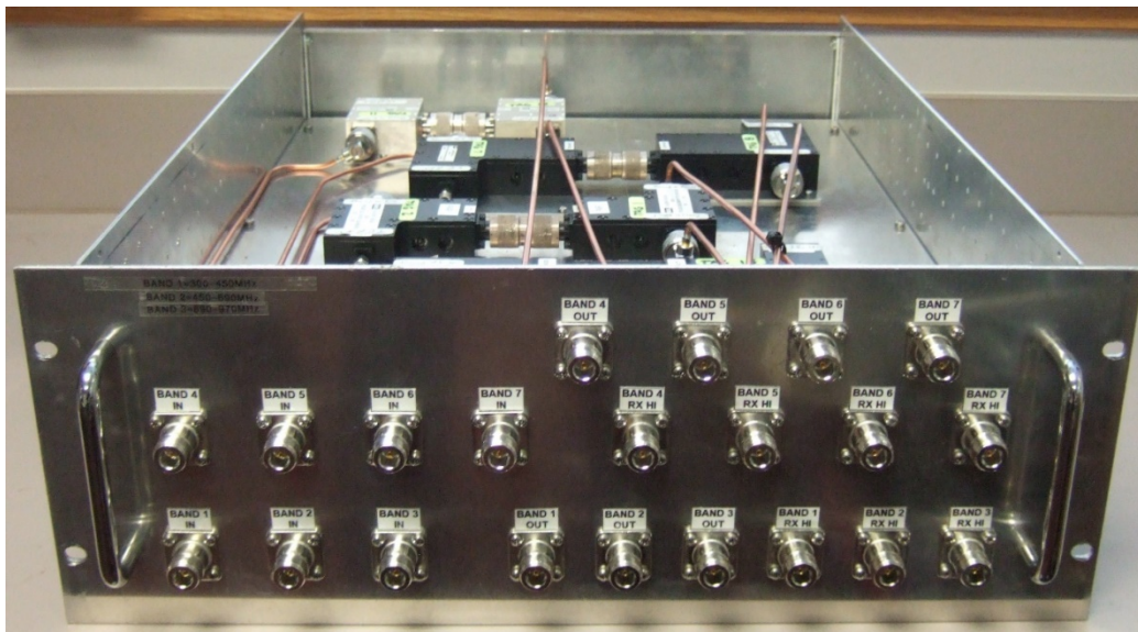
Fig. 9 Front panel for the rack-mount box seen in Fig. 8. Each band has three ports: “IN”, “OUT”, and “Rx-Hi”. For Tx mode, the ports are connected externally as in Fig. 6. For Rx mode, the ports are connected externally as in Fig. 7.
