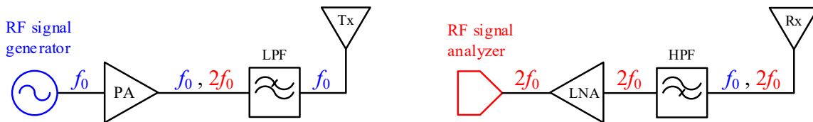
Fig. 2 Passive filtering implemented in the transmitter after the power amplifier (PA) (lowpass) and in the receiver before the low-noise amplifier (LNA) (highpass)
