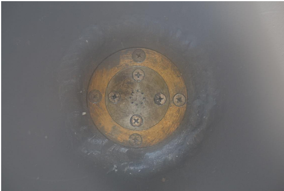
Fig. 10 Flush mount pressure gauge installed in an ammo compartmentation experiment
