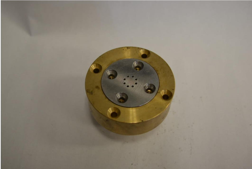
Fig. 8 Assembled inner components of the mount and gauge
