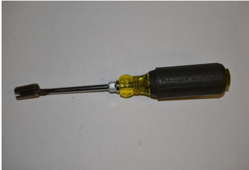
Fig. 9 Gauge installation tool
