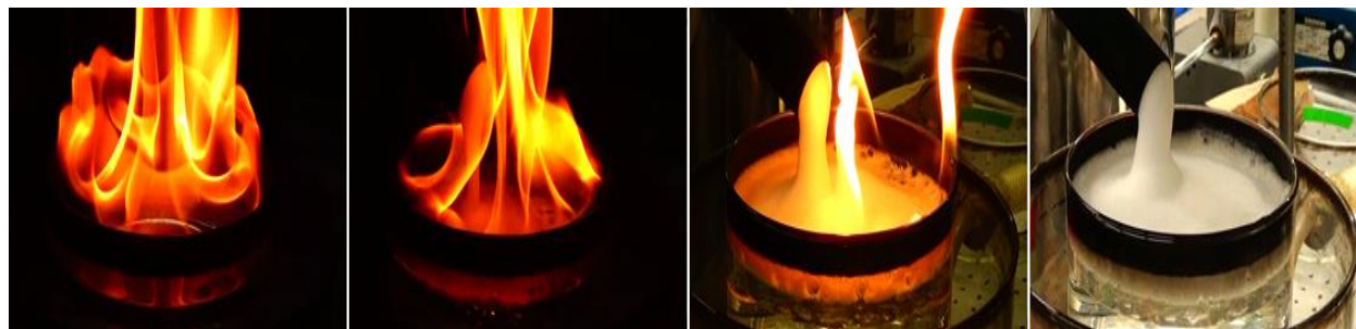
Figure 39. A pool (12-cm diameter, n-heptane liquid, 2-cm lip) fire extinction by foam applied at the center at a constant flow rate; from 30-sec pre-burn to extinction.
