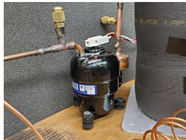
Proof of concept for miniature compressor-based cooler.
