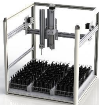
Concept drawing of modified liquid handler with standard vial racks
