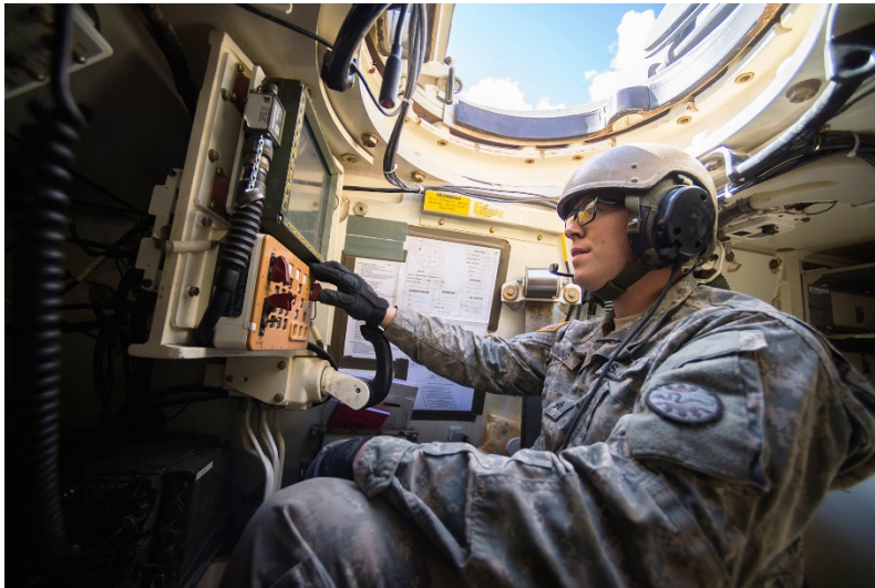
Fig. 2 Military combat vehicle crew tank helmet headset with radio intercom embedded (photo credit: US Army, Sgt. Mason Cutrer https://www.defense.gov/observe/photo-gallery/igphoto/2002137607/ )
