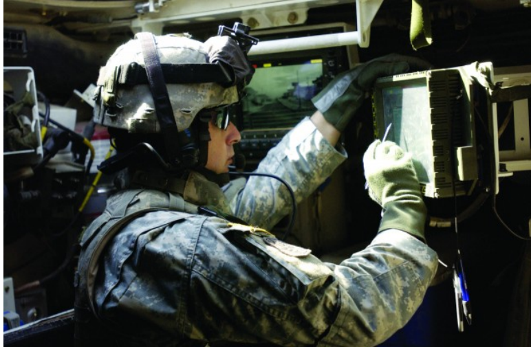
Fig. 4 Example of monitors in a combat vehicle (Center=CITV; Right=FBCB2; photo credit: US Army: https://www.army.mil/article/63135/army_links_tactical_radios_chat_services_with_commercial_communications )
