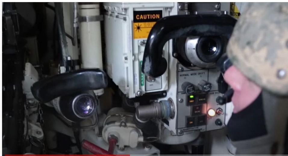
Fig. 7 Example of the M1A2 gunner's station (photo credit: US Army images by Spc J Hester-Heard, https://www.youtube.com/watch?v=KW2YMnD3HYk )
