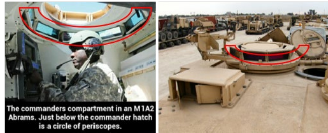
Fig. 10 Vision blocks highlighted in red (left=from the inside; right=from the outside)
