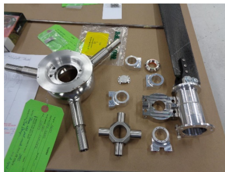
(a) isolated blade (b) blade and gimbal hub (c) 4-axis Tormach mill Figure 2. Tiltrotor blade shown with parts of the new gimbal hub.
