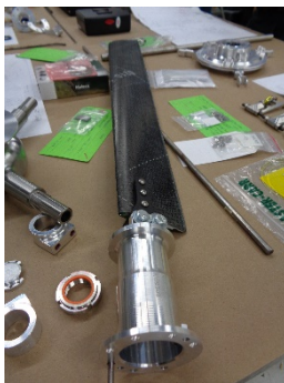
(a) isolated blade (b) blade and gimbal hub (c) 4-axis Tormach mill Figure 2. Tiltrotor blade shown with parts of the new gimbal hub.
