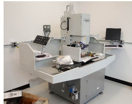
(a) isolated blade (b) blade and gimbal hub (c) 4-axis Tormach mill Figure 2. Tiltrotor blade shown with parts of the new gimbal hub.
