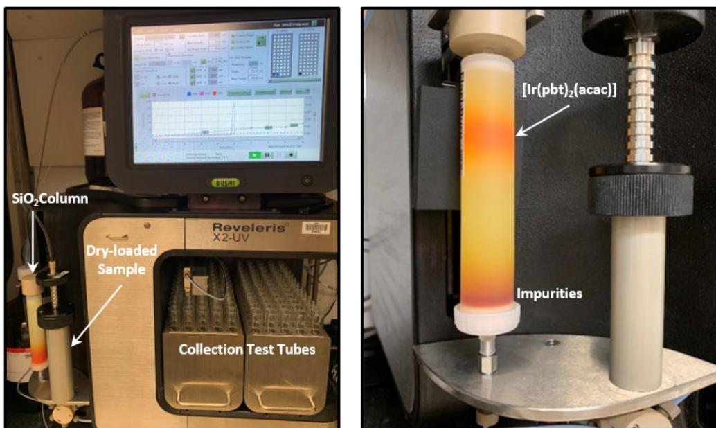
Fig. 6 (left) Reveleris running a column chromatography process. (right) Close-up of silica column showing the bright orange band associated with pure  $[\text{Ir}(\text{pbt})_2(\text{acac})]$ .
