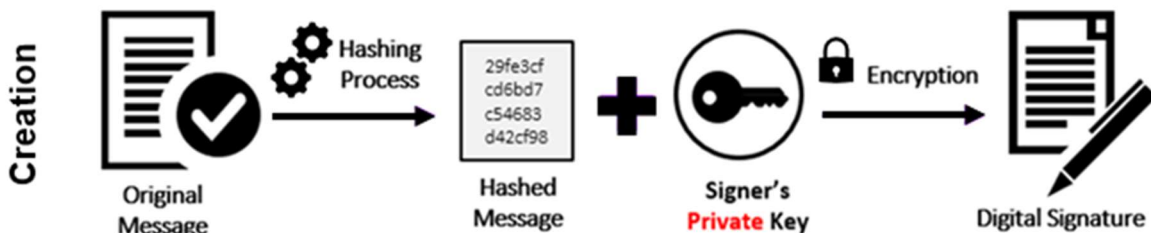
Figure 8. Digital Signature Creation Using Hashing and a Private Key
