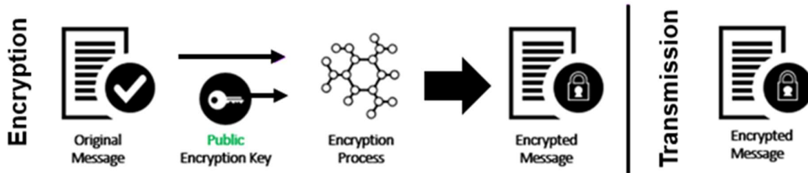
Figure 4. Encryption using Asymmetric Key Encryption
