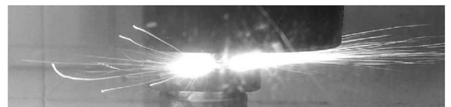
Fig. 20. Violent exothermic reaction of Al-PTFE during quasi-static compression [137].
