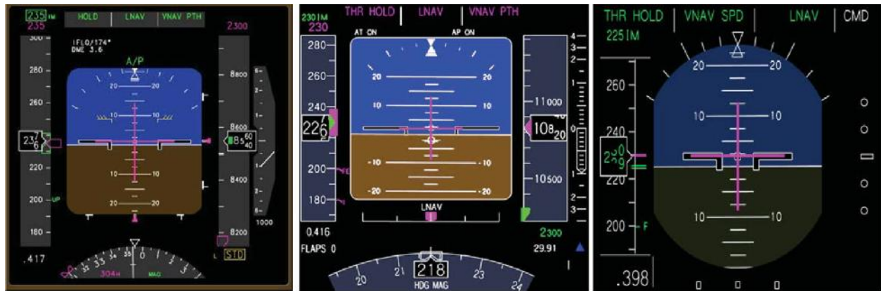
Figure 2-22. PFDs with IM Features from Baxley et al. (2013) [Reprinted from Baxley et al., 2013]
