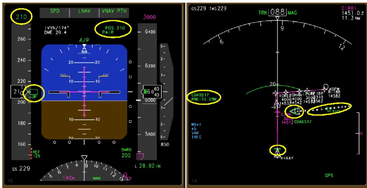
Figure 2-19. PFD and Navigation Display with IM Features from Barmore et al. (2005) [Reprinted from Baxley et al., 2014 (Highlights Added)]
