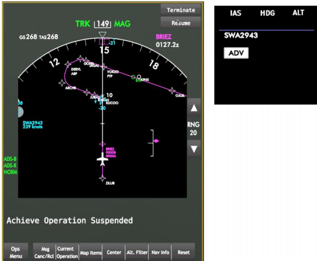
Figure 3-14. CDTI Traffic Display and AGD During Suspend State
