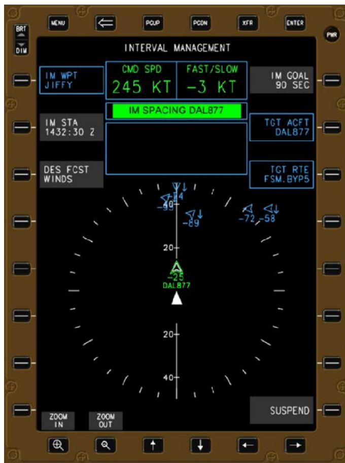
Figure 2-25. CDTI Traffic Display with IM Features from Kibler et al. (2015) [Reprinted from Kibler et al., 2015]
