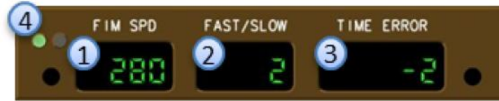
Figure 2-28. Numeric AGD with IM Features from Swieringa et al. (2014) [Reprinted from Baxley et al., 2014]
