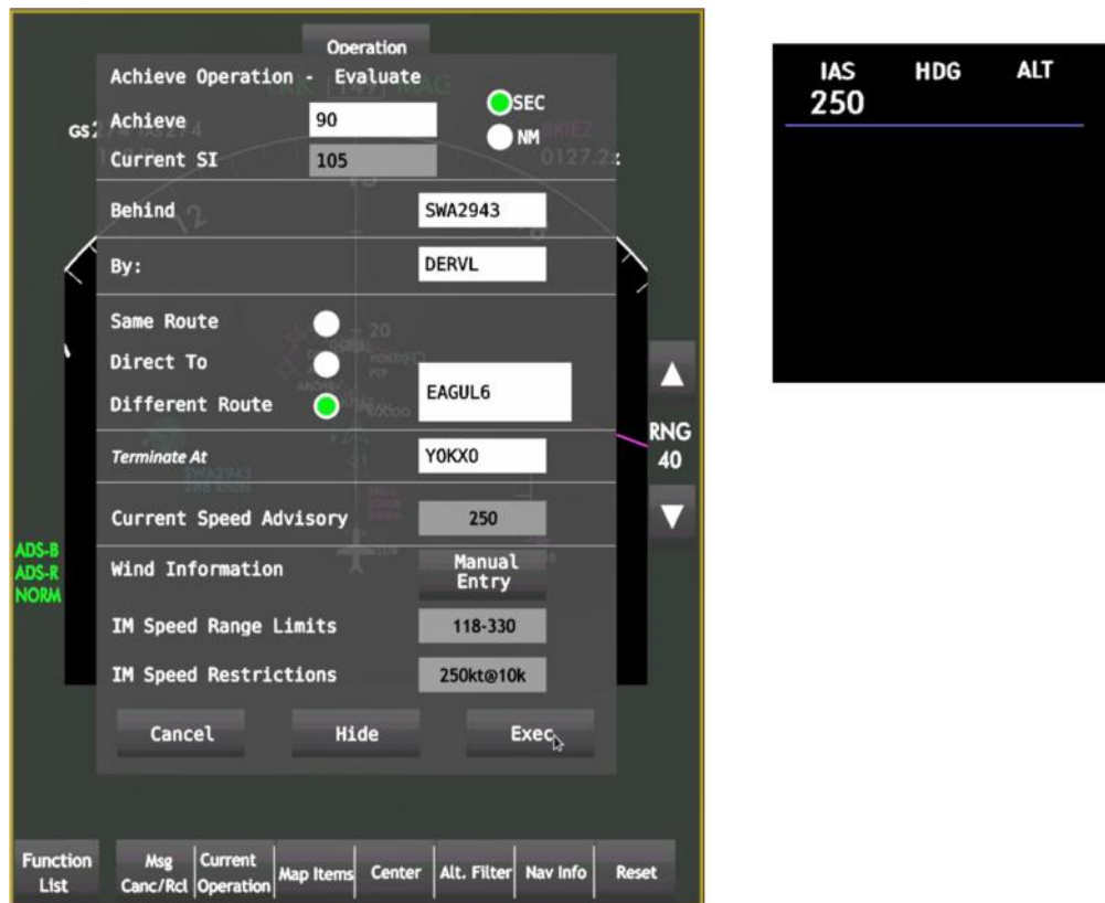
Figure 3-10. CDTI Traffic Display and AGD During Evaluate State
