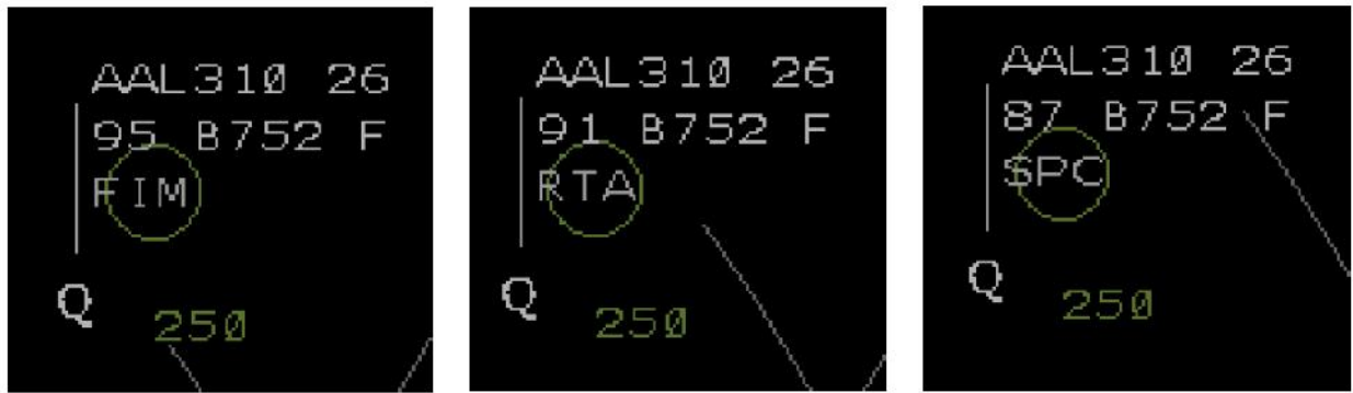
Figure 2-12. TRACON Controller Data Block Information from Callantine et al. (2013) [Reprinted from Callantine et al., 2013]
