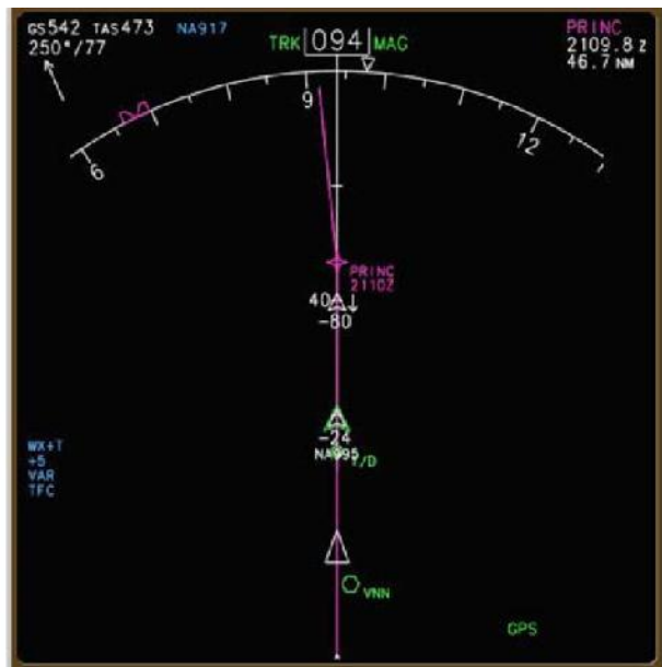
Figure 2-20. PFD and Navigation Display with IM Features Implementation 1 from Murdoch et al. (2009) [Reprinted from Baxley et al., 2014]
