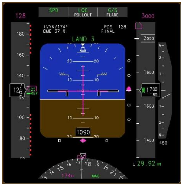
Figure 2-20. PFD and Navigation Display with IM Features Implementation 1 from Murdoch et al. (2009) [Reprinted from Baxley et al., 2014]
