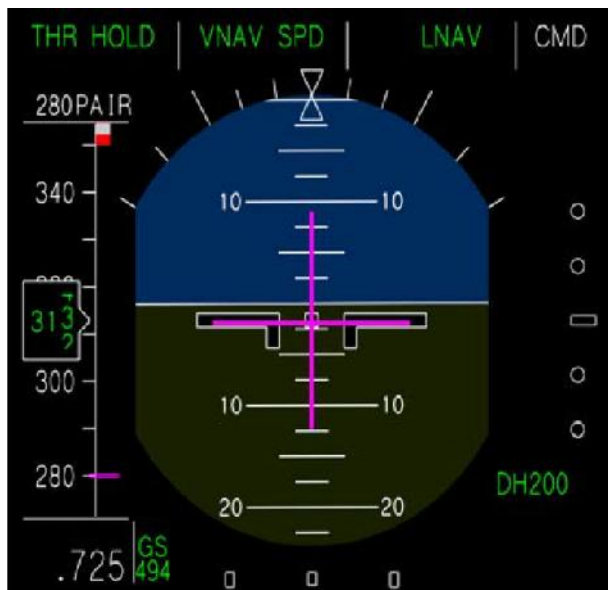
Figure 2-21. PFD and Navigation Display with IM Features Implementation 2 from Murdoch et al. (2009) [Reprinted from Baxley et al., 2014]
