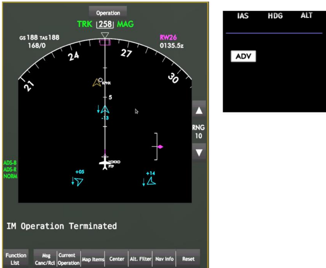
Figure 3-15. CDTI Traffic Display and AGD During Terminate State
