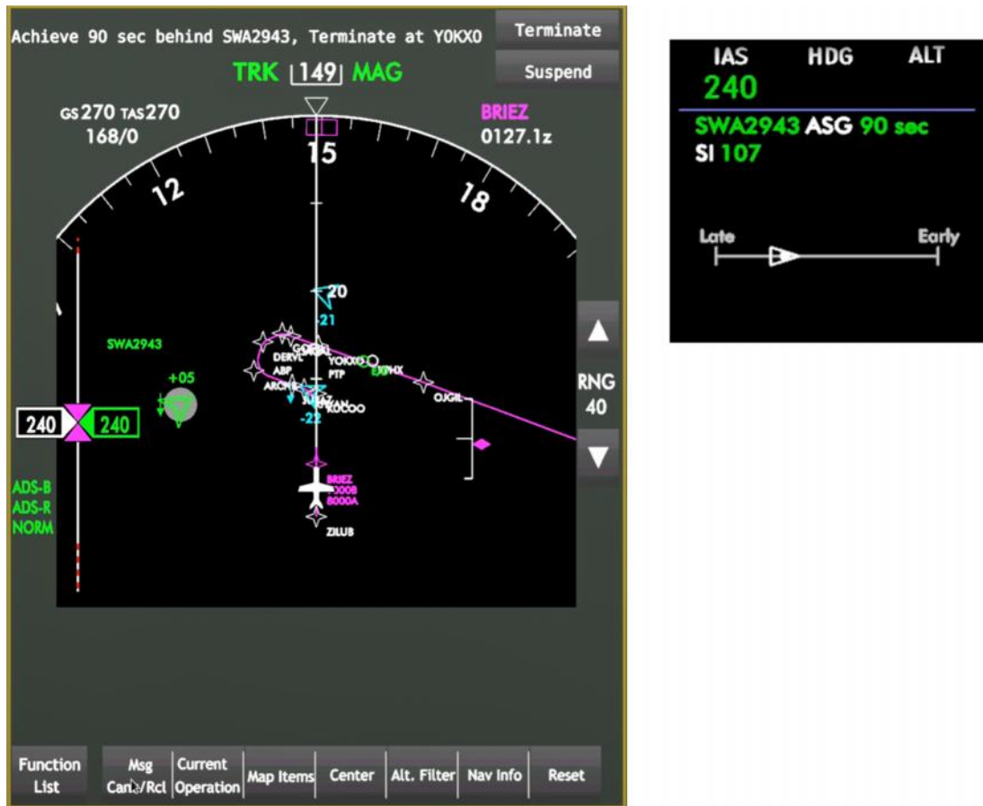
Figure 3-11. CDTI Traffic Display and AGD During Execute State
