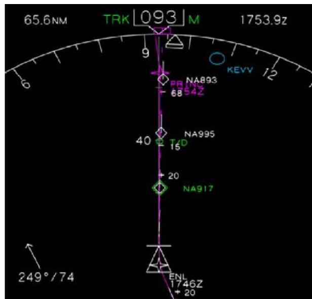
Figure 2-21. PFD and Navigation Display with IM Features Implementation 2 from Murdoch et al. (2009) [Reprinted from Baxley et al., 2014]
