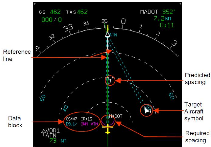
Figure 2-14. Navigation Display with IM Information from Hebraud, Hoffman, Papin et al. (2004) First Evaluation [Reprinted from Hebraud, Hoffman, Papin et al., 2004]
