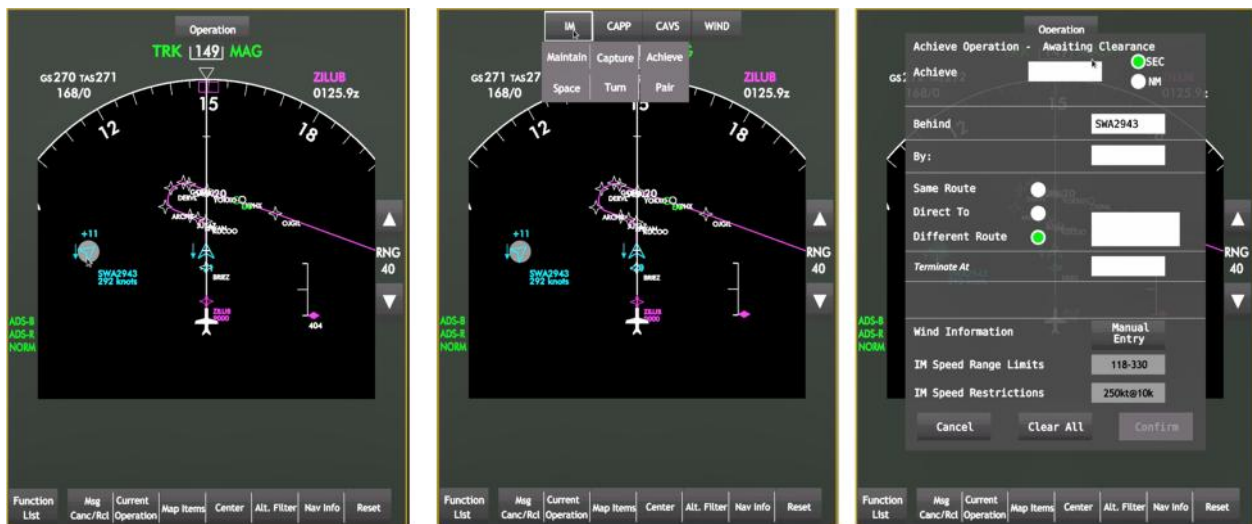
Figure 3-9. CDTI Traffic Display and AGD During Awaiting Entry State
