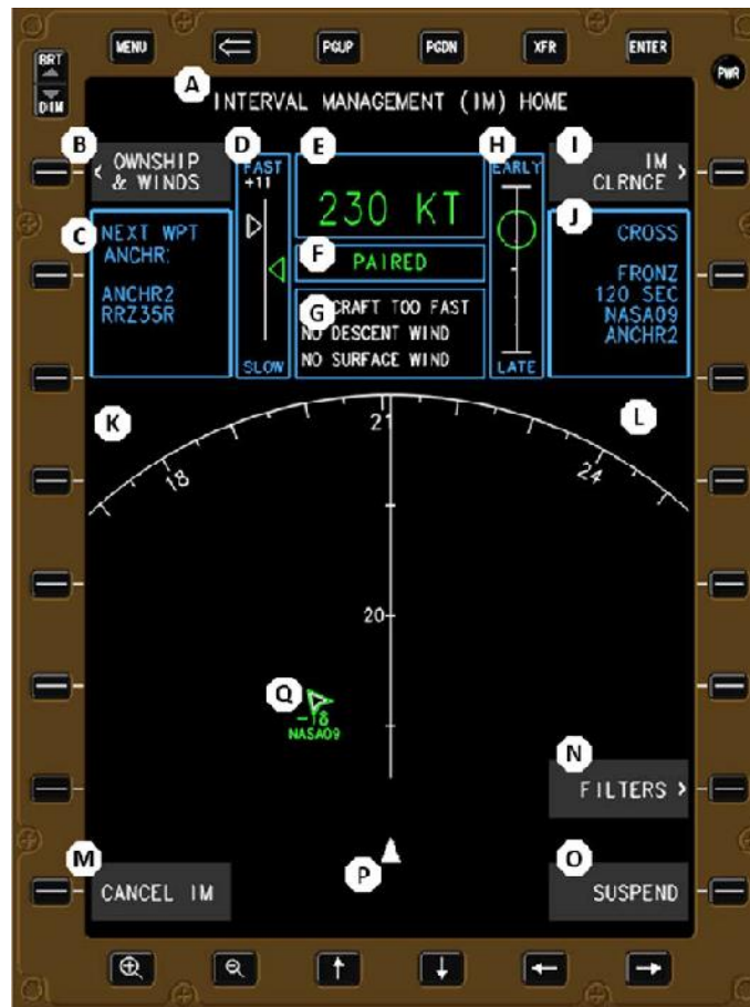
Figure 2-30. CDTI Traffic Display with IM Features from Baxley et al. (2016) [Reprinted from Baxley et al., 2016]
