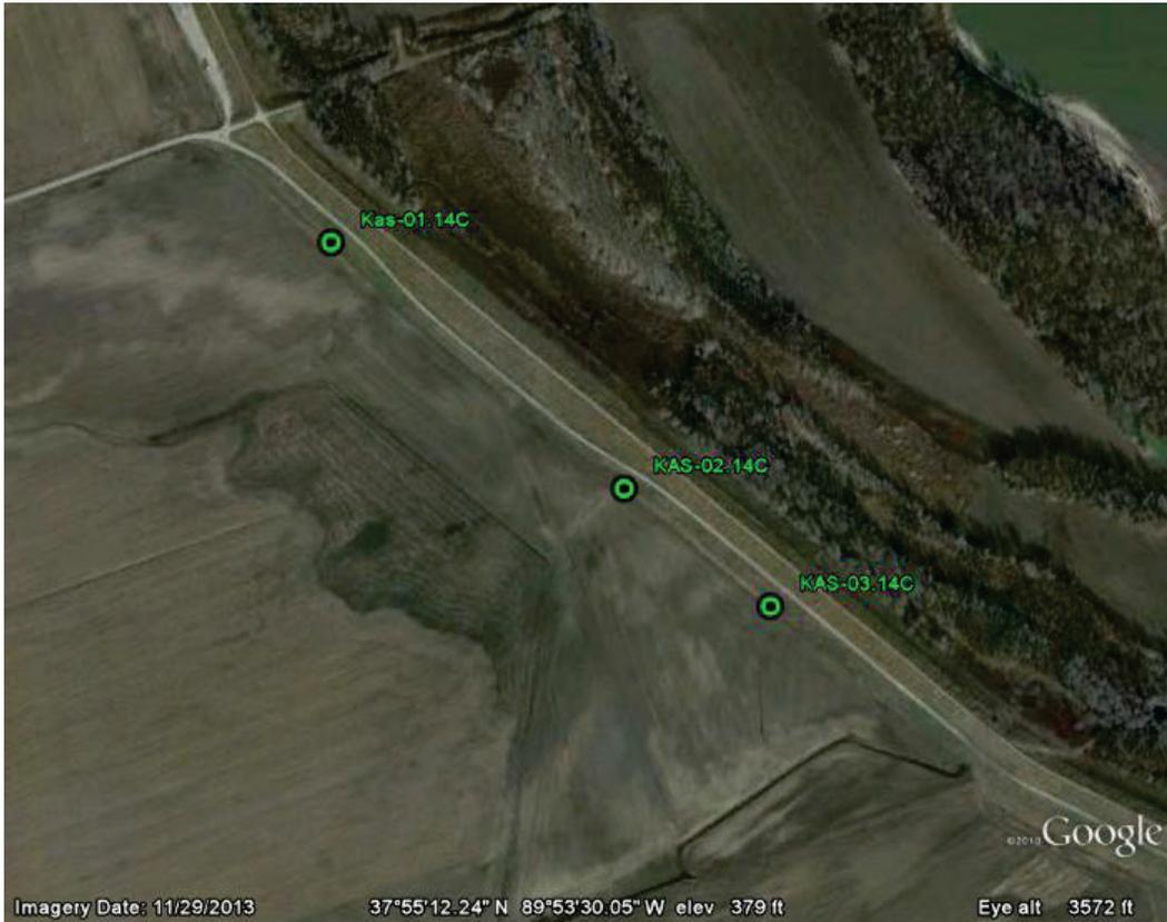
Figure 23. CPT sounding locations near Sand Boil (SB) No. 1 (yellow) and within designated study area No. 2.
