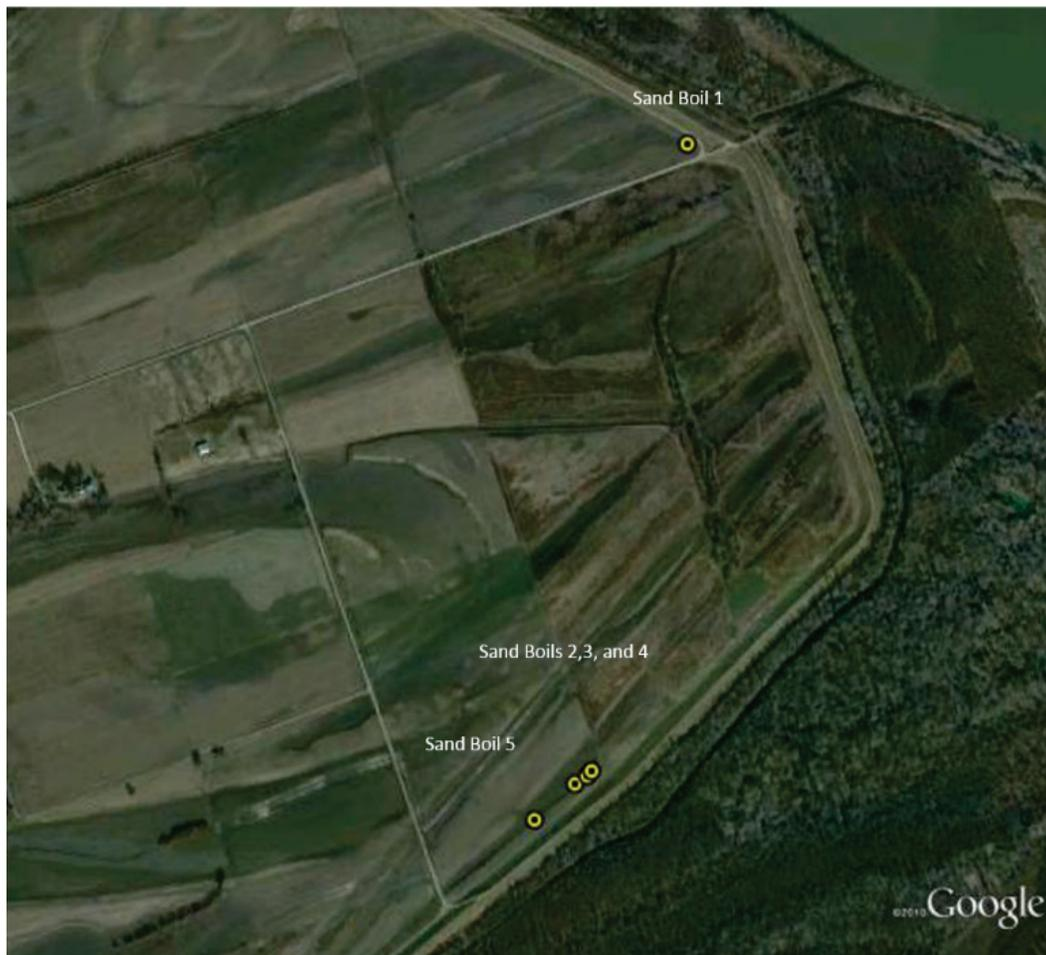
Sand boil location and relevant characteristics were collected using a GeoXH 6000 handheld global positioning system (GPS) device and the Mobile Information Collection Application (MICA) software. Measurements of cone height and inside throat diameter were recorded.
