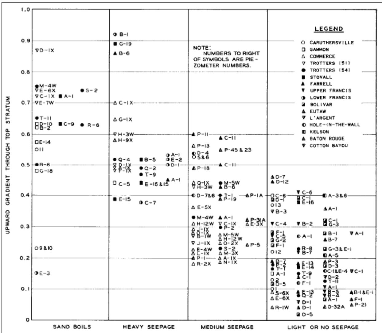
In addition to the hydraulic gradient and the blanket thickness, material properties of the blanket itself have a direct bearing on seepage and sand boil potential. The gradient required to cause heaving and possible fracturing of the top stratum is defined as the *critical gradient* and corresponds to the ratio of the submerged unit weight of the soil comprising the top stratum and the unit weight of water (Turnbull and Mansur 1961).
