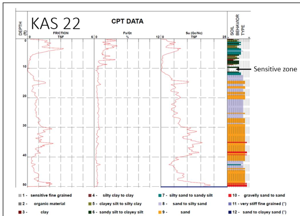
KAS-22 was continuously sampled from the surface of the berm to 3 ft into the top of the alluvial aquifer. The berm and blanket were composed of silt and clay with sand (Table 2), which is consistent with the CPT log in Figure 63. A sensitive zone composed of wet, soft, silt (ML) is present at the top stratum and substratum interface.
