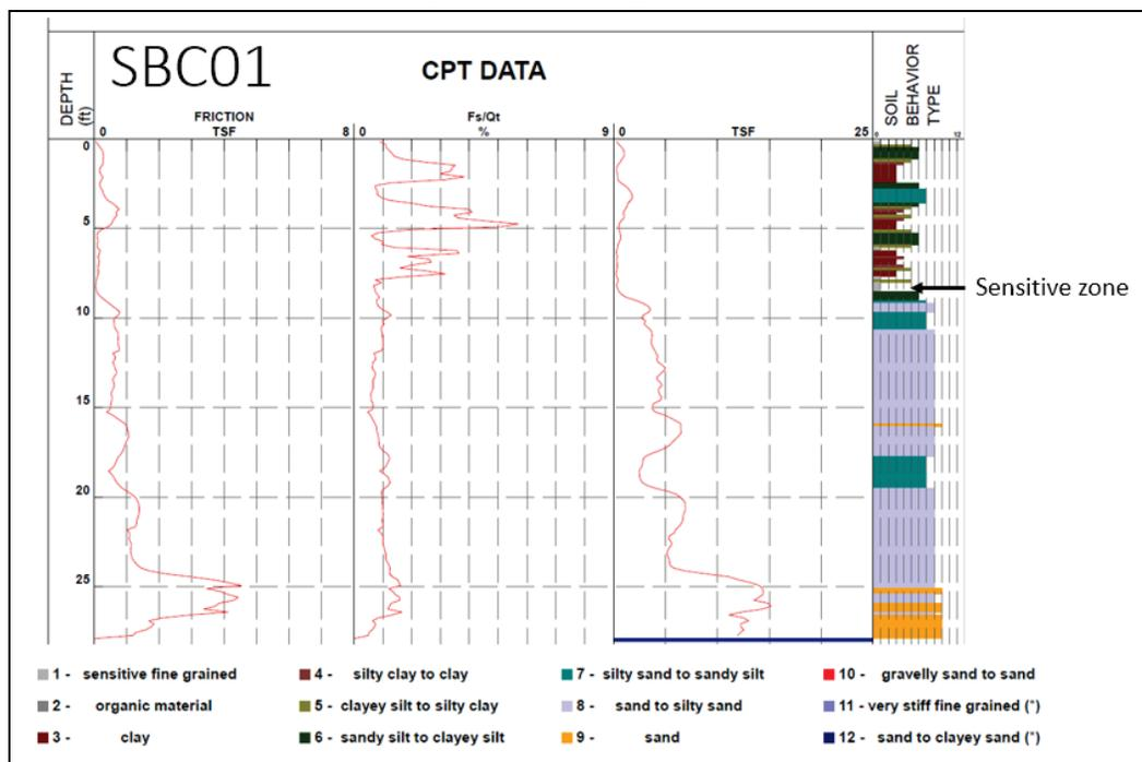
The sensitive zone was sampled between 8.5 and 10 ft and was composed of wet, soft, silt (ML). A cross section presented previously as Figure 57 identifies this zone in profile and relationship to the underlying aquifer sands and the blanket.
