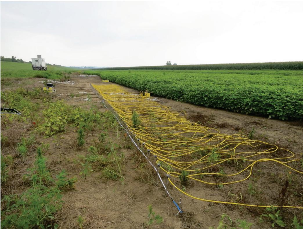
The 14 ERT surveys were conducted in three groupings (Figures 36 and 37) within a larger area (approximately  $125 \times 30$  m, or approximately  $410 \times 100$  ft) that had most recently experienced sand boil activity during the summer of 2013. All ERT surveys were collected on the landside of the Kaskaskia levees.
