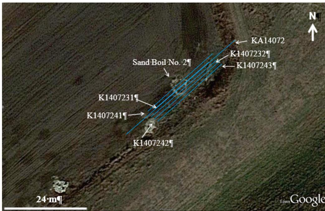
Figure 42. ERT File KA140722. Representative ERT inversion results for Sand Boil No. 2 identifying three major stratigraphic layers. Electrode spacing 0.5 m.
