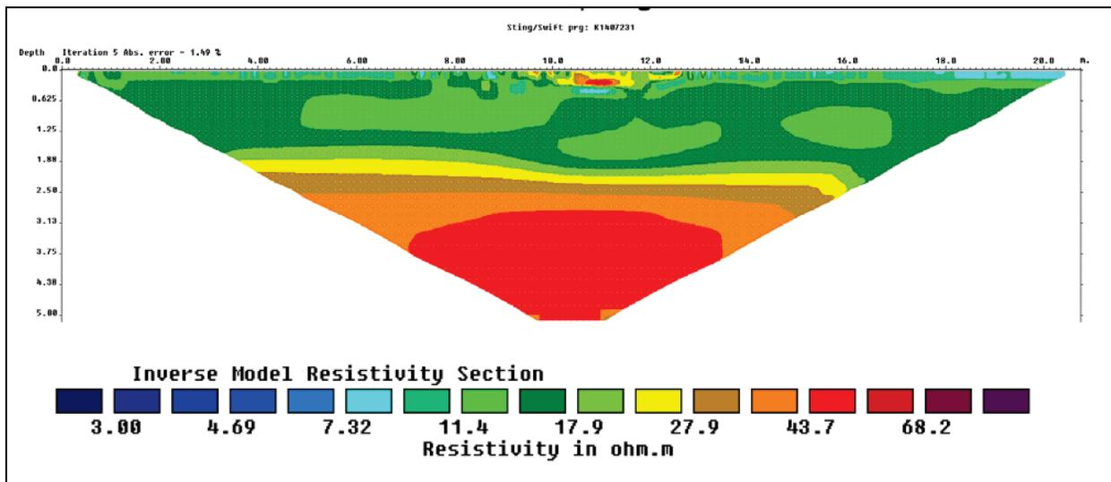
Both of the resistivity sections shown in Figures 42 and 43 identify an area of higher resistivity at the location of the sand boil to a depth of  $\sim 0.6$  m. Survey K1407231 depicted in Figures 43 and 44 used an electrode spacing of 0.25 m. The measured values clearly show much higher resistivity (27 to 50 Ohm-m) below the boil area than the surrounding top stratum not immediately affected by the sand boil.
