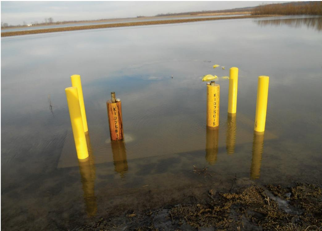
The KAS-14-201C piezometer at the levee toe is used here as a proxy to estimate the landside head and the value for  $h_o$  by the above equation
