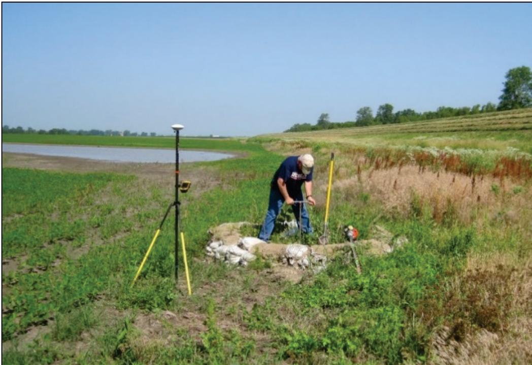
A second gal-sized soil sample was taken from the blanket material nearby. Both samples were wrapped in plastic and sealed for transport to ERDC for particle-size analysis and mineralogy. Results of the laboratory testing of the ejecta and blanket samples are presented in Table 1. Curves of the grain-size data from laboratory testing of these samples are presented in Appendix A.
