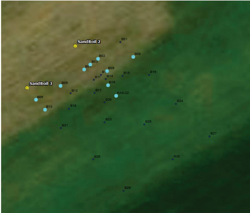
Figure 61. G series CPTs containing sensitive fine-grained layer (cyan highlighted).
