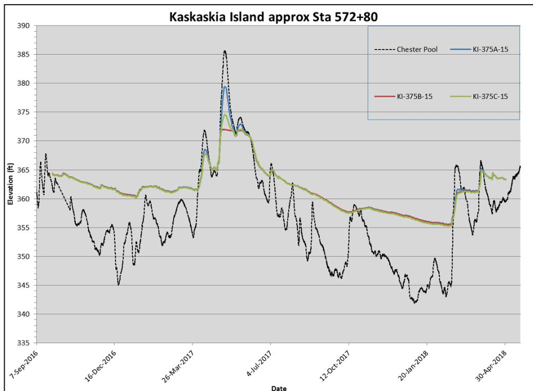
For 575B and 575C wells, the calculated groundwater responses were at elevation 376.27 ft and 376.54 ft, respectively. These groundwater levels correspond to a value of  $h_o$  in a hypothetical standpipe of 7.38 and 7.81 ft above the ground surface at these well locations. The exit gradient for these locations with a 10-ft-thick blanket and no tail water was 0.738 and 0.781 for the 575B and 575C wells, respectively.
