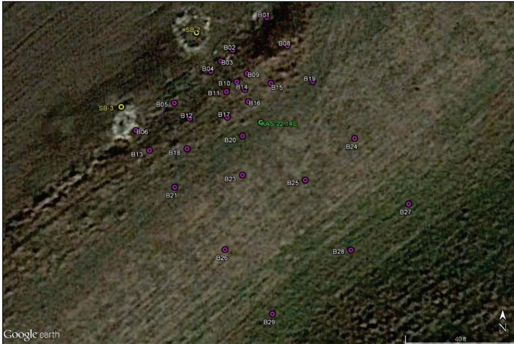
Figure 26. Close-up view of CPT sounding locations in slump (depression) area.
