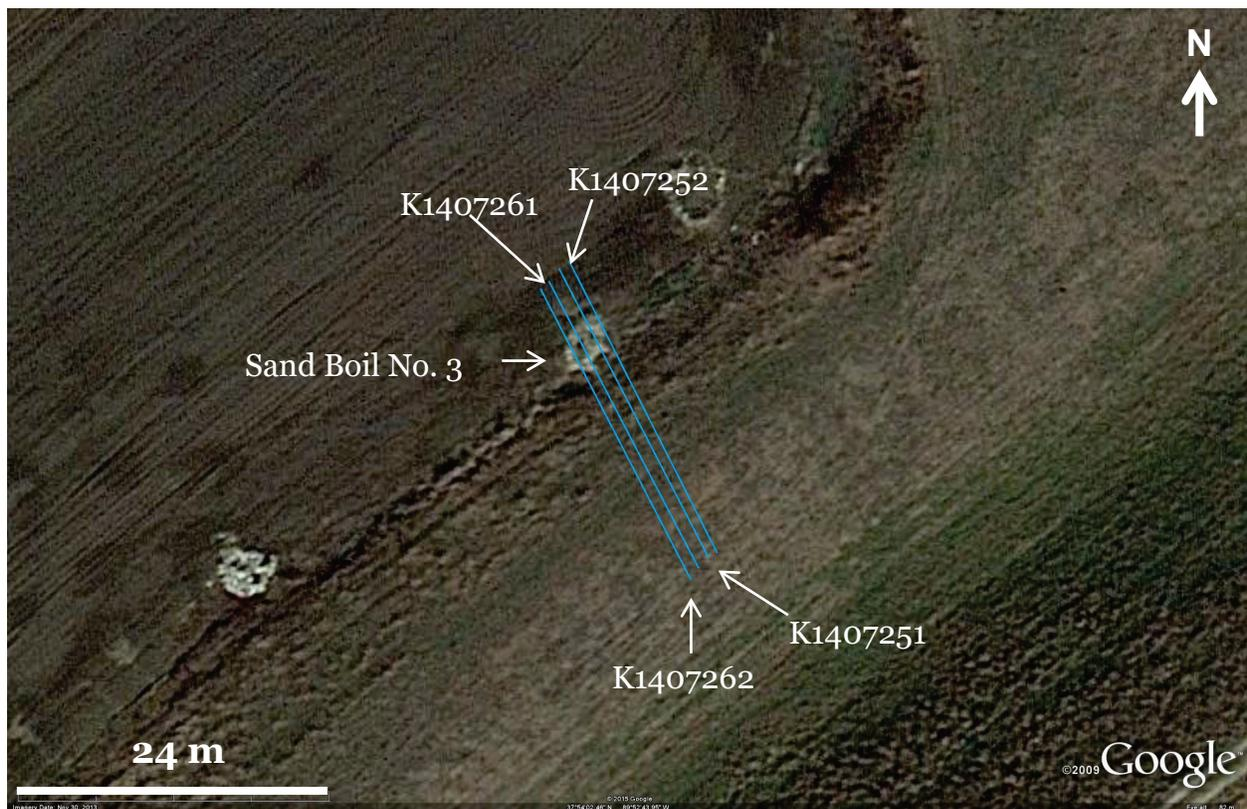
A representative resistivity section from these four surveys is presented in Figure 46 (profile K1407262). Inversion results show noticeable disturbance of the top stratum directly below the boil area, which is ~5 m wide and 2 m deep. The area affected by the sand boil has a much higher resistivity signal than the surrounding top stratum soil, corresponding to the green-colored layer, with resistivity values of 8 to 10 Ohm-m in Figure 46.
