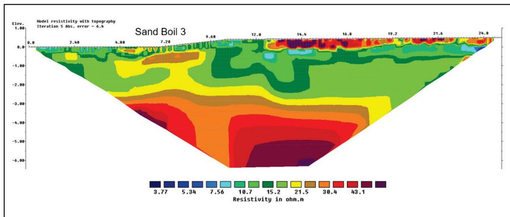
The resistivity profile in Figure 46 extends onto the seepage berm and is interesting because of the presence of a resistive ( $>30$  Ohm-m) layer at the surface. The levee designers intended for the berm to be pervious as evidenced by the nearly 1 m (3 ft) of resistive soils (sands) overlying the top stratum (or blanket) foundation beneath the levee. A common practice to control underseepage at the landside levee toe was the addition of a pervious seepage berm (USACE 1956a, 1956b; Moore 1972).
