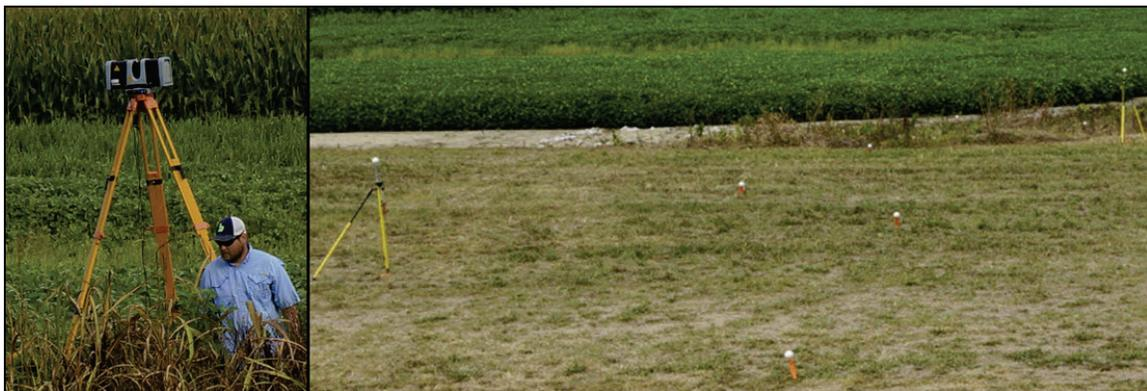
The laser was initialized and a small mirror within the instrument began to spin, which in turn pulsed the laser beam as far as it can “see,” capturing up to 200,000 data points per second. The collection was complete for that station once the instrument had completed the full 360 deg rotation. A data gap or shadow occurred underneath the
