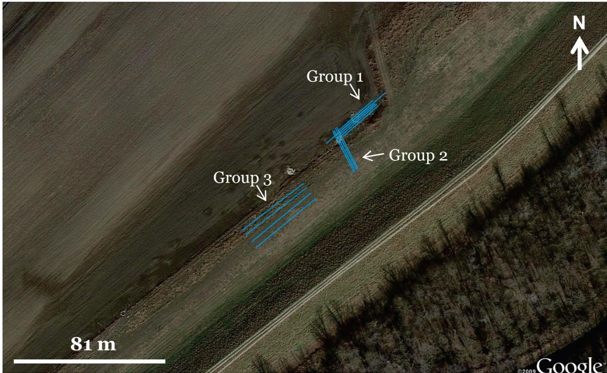
Figure 37. Location of ERT surveys relative to the levee, berm, and farm fields.
