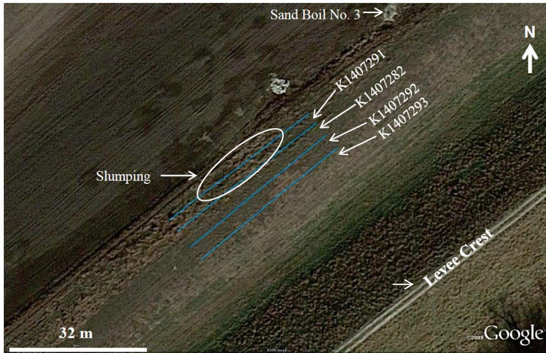
Figure 48. ERT File K1407292 ERT survey along berm near slump area.
