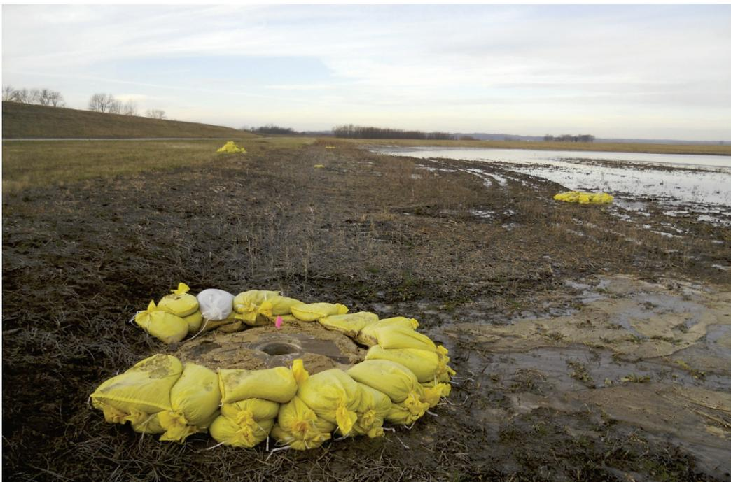
Figure 72. Close-up view of the 4.3-ft-diam sand boil cone at sand boil No. 151, with nearly a 12-in.-diam throat. Boil was no longer active as the river fell below a critical threshold on 5 Jan 2016 visit.
