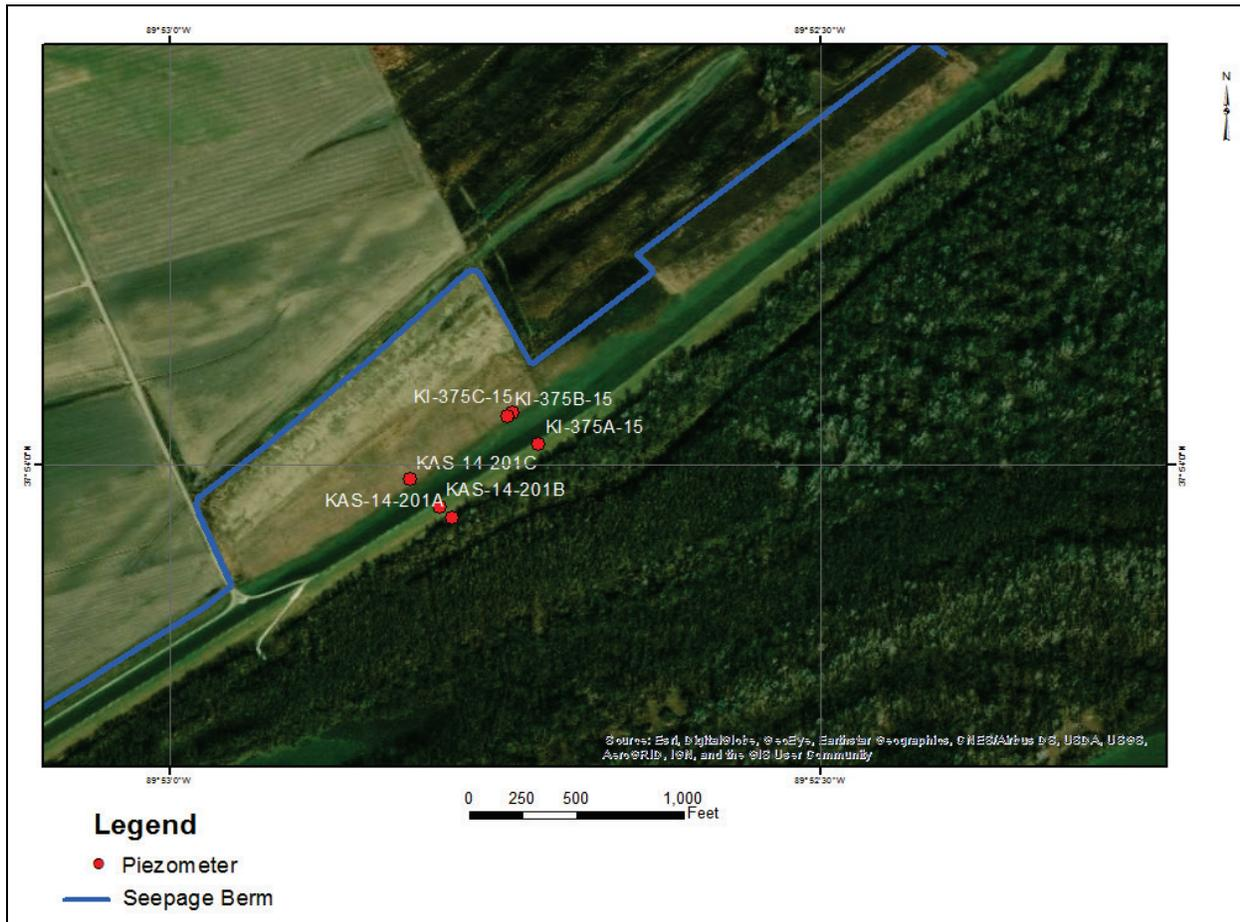
The record of daily groundwater elevation in the landside toe well (KAS-14-201C) easily permits the exit gradient at this location to be estimated for the 2013 Flood conditions by inference from a flood of similar stage comparable to that occurring in 2013.
