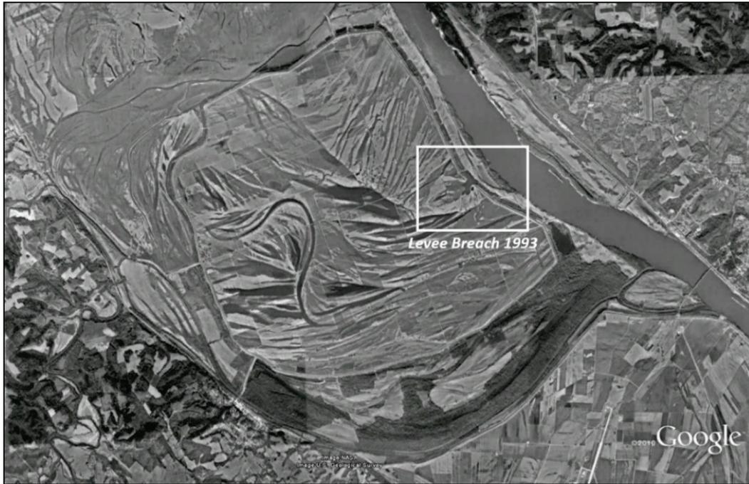
Figure 9. Floodwater in farming area on Kaskaskia Island in 1993 after levee breach. (Photo courtesy of St. Louis District.)
