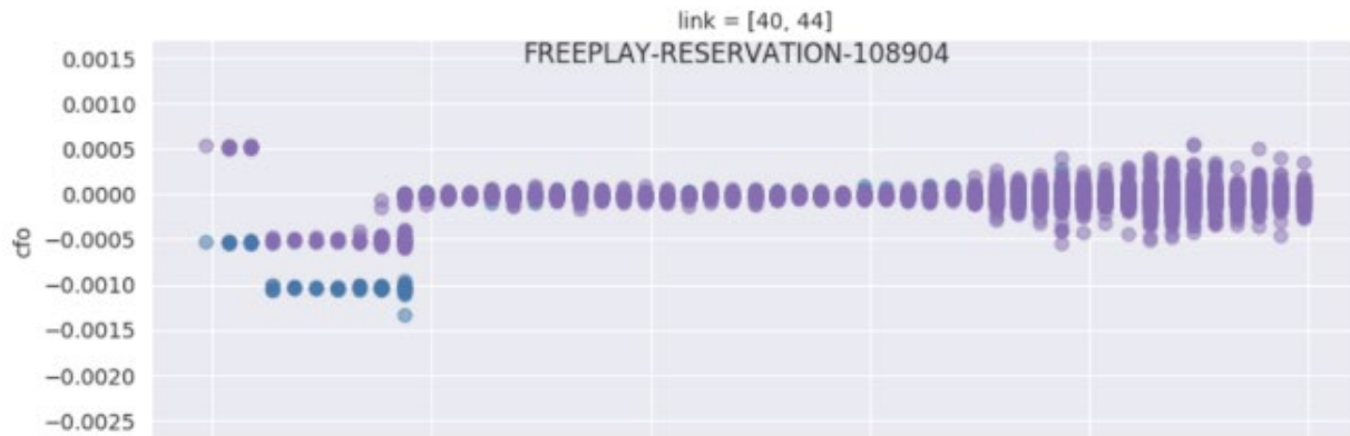
Figure 11 Trajectory of the carrier frequency offset over time
