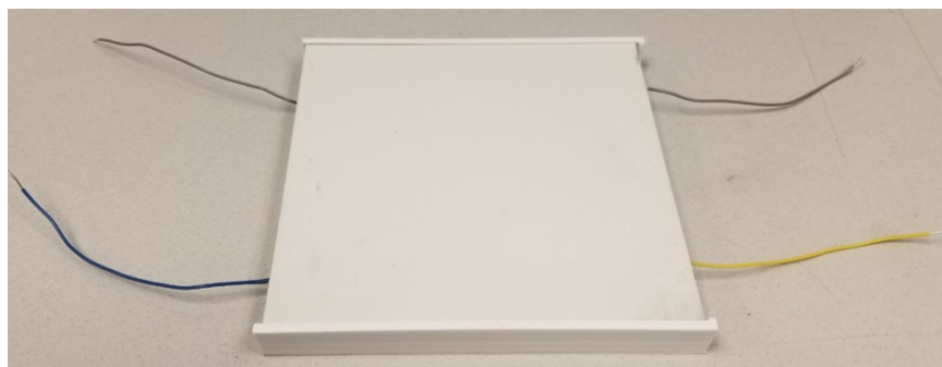
Figure 4.12: Photograph of the stacked-up multilayer absorber (with the plasma-shells embedded within the lossy magneto-dielectric) inside the 3D printed frame.
