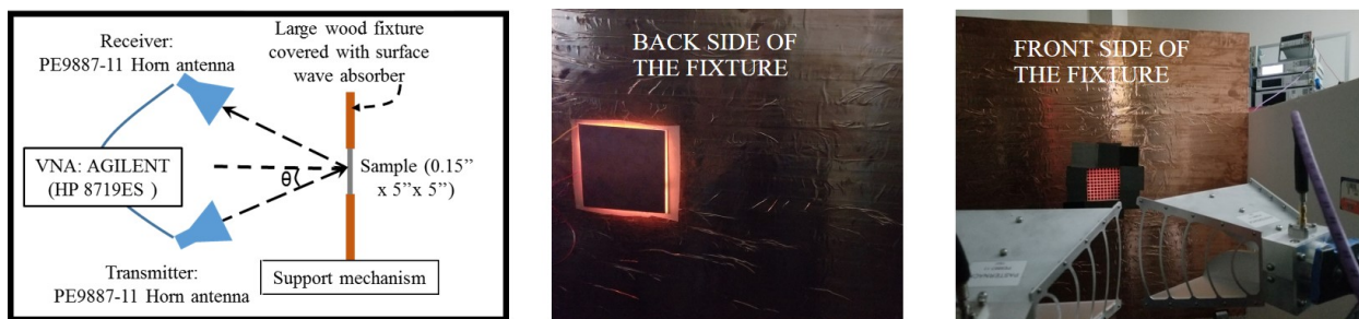
Figure 3.11: Sketch and photograph of the test setup (free space) for the absorber measurement.
