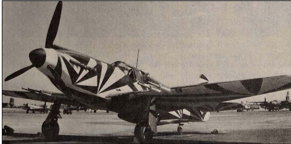
Figure 34: P-51 Dazzle-Design Experiment in WWII
