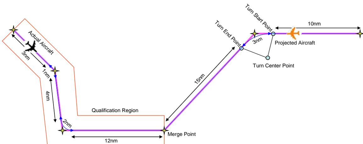
Figure 1. Illustration of RPI Application
