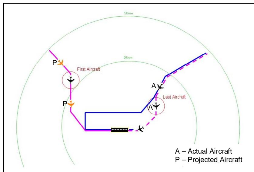
**Figure 9. Runway Change Application of RPI: Indication of Relative Sequencing of Flows**
