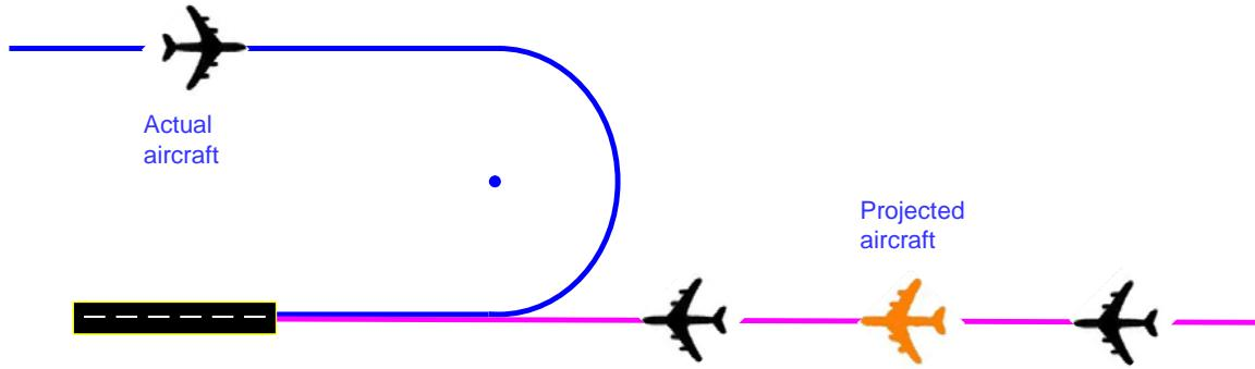
**Figure 2. RPI Application with RF Leg**
