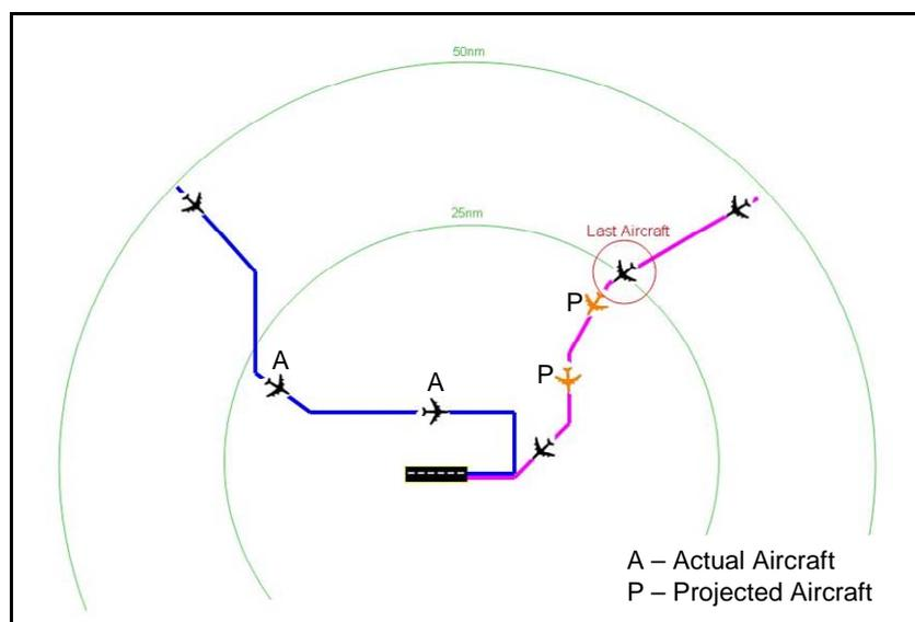
**Figure 8. Runway Change Application of RPI: Identification of 'Last Aircraft' in Flow**
