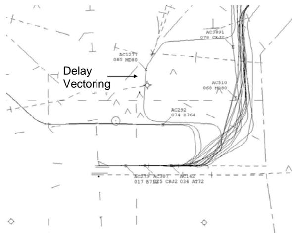
**Figure 4. Delay Vectoring**
