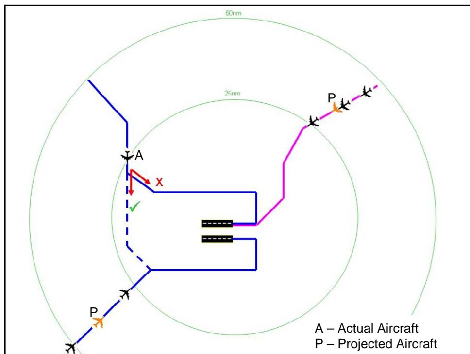
**Figure 7. Illustration of TMC Decision to Flow Aircraft Using RPI**
