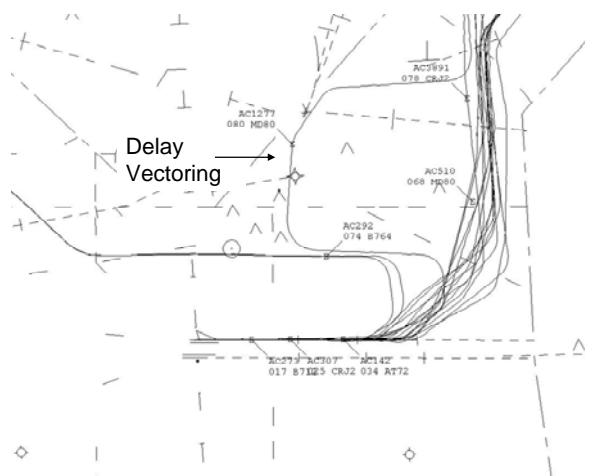
**Figure 4. Delay Vectoring**
