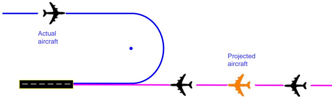
**Figure 2. RPI Application with RF Leg**
