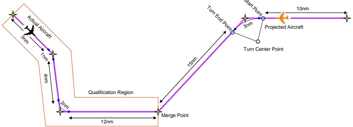
**Figure 1. Illustration of RPI Application**
