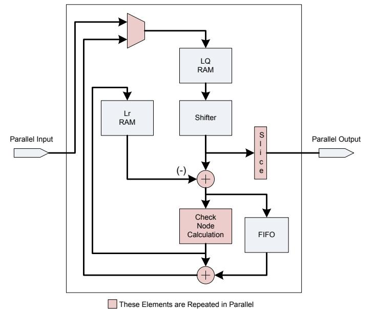
Figure 3. Decoding Core
