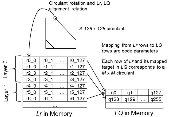
Figure 1. An example decoder memory layout of  $Lr$  and  $LQ$  for a hypothetical code with circulant size of  $M = 128$ . Each map from a row of  $Lr$  to a row of  $LQ$  corresponds to a circulant in the parity check matrix. The relation of the circulant rotation and the left rotation of a  $LQ$  row to align with the  $Lr$  row is indicated.
