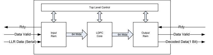
Figure 7. Decoder Top Level Diagram
