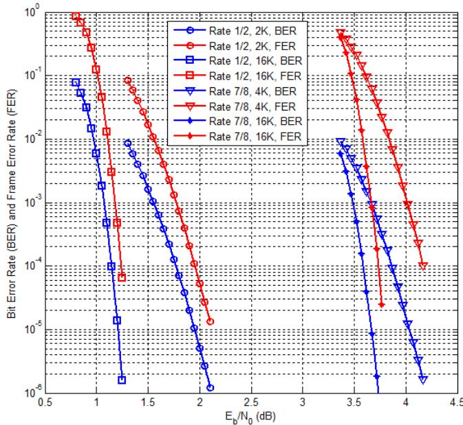
Figure 8. Simulated BER and FER curves for the four implemented codes using a fixed point decoder model running at 30 iterations.
