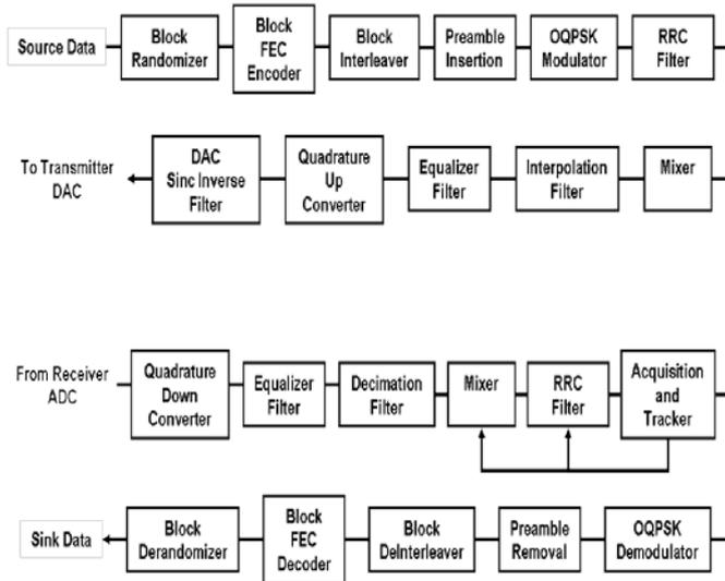
Figure 6 Components of the Test Waveform
