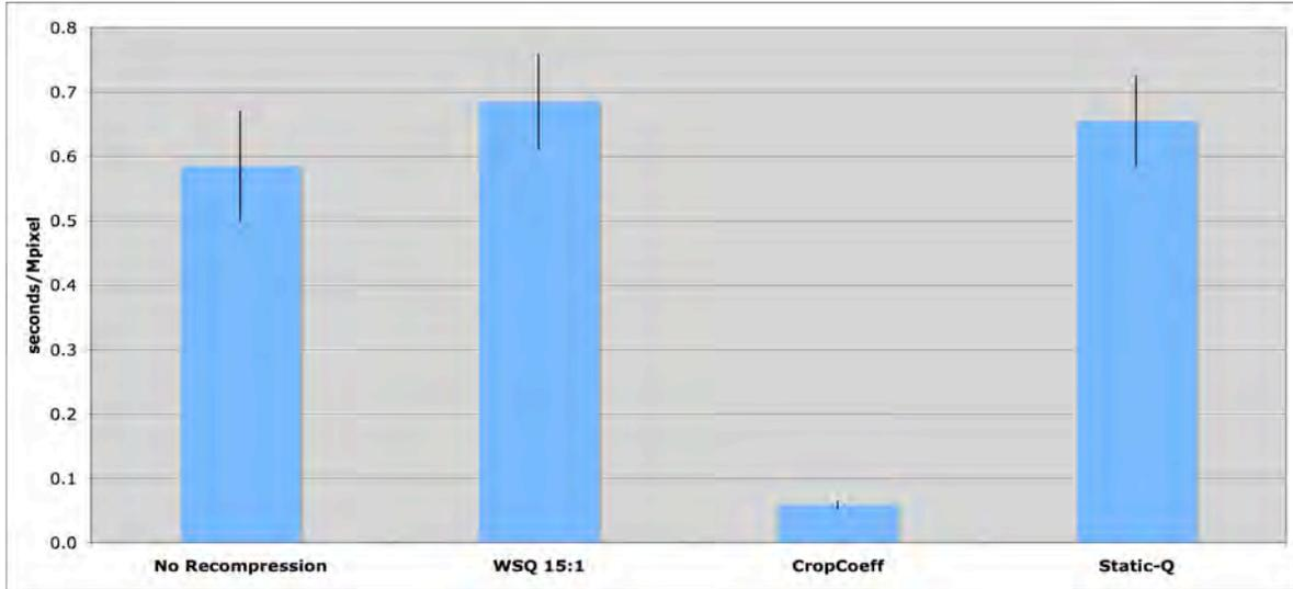
**Figure 3.** Computation time by recompression type. Error bar =  $1\sigma$ .
