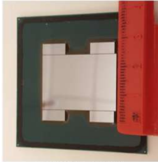
(a) Delidded Stratix 10 FPGA
