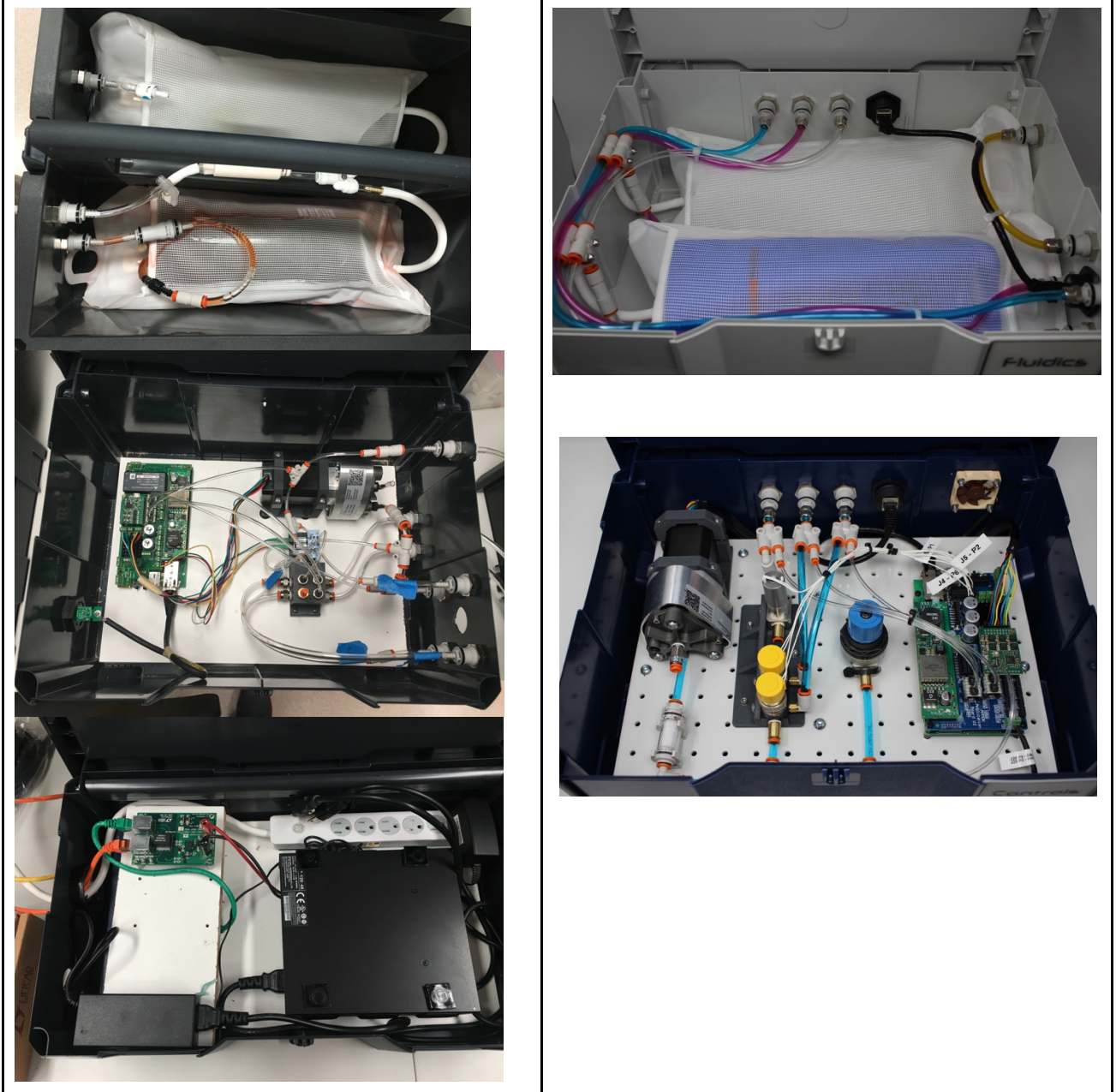
Figure 51: As shown by the internal components of the fluidics supply stacks, the beta prototype has decreased the amount of space needed by moving the Wi-Fi router and power supplies from the stack. Furthermore, the hoses do not route the full 4 L of fluids, but also provides a loop back through the fluidics box for waste (yellow tubing).
