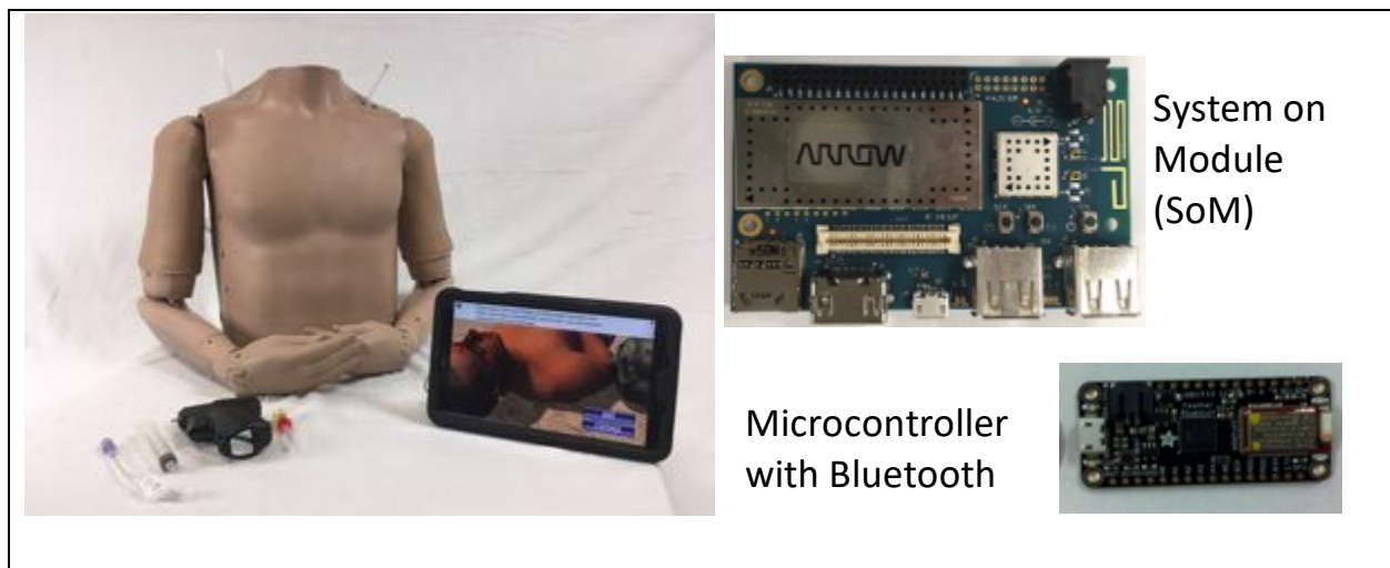
Figure 55: The BRMTS implements the AMM Core on a credit card-size computer embedded in the HHIO trainer.
