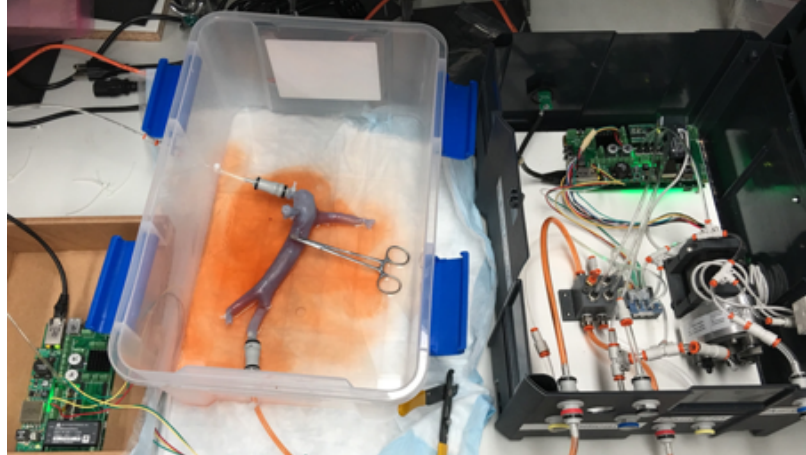
Figure 26: Mule I Integration: Bleeding Vena Cava prototype module connected to Fluidics system, both running on identical sets of AMMDK CCB & Application Boards.
