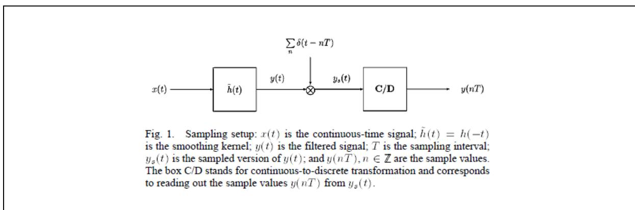
Figure 1 - FRI Block Diagram from [4]
