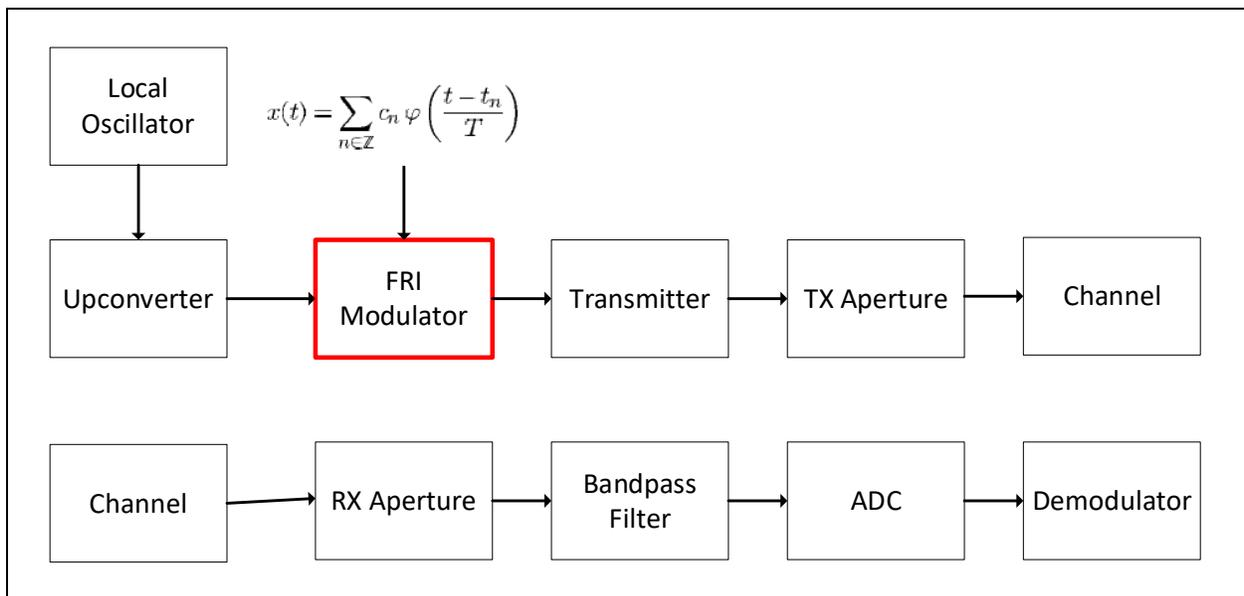
Figure 2 - RF FRI Communications System Block Diagram
