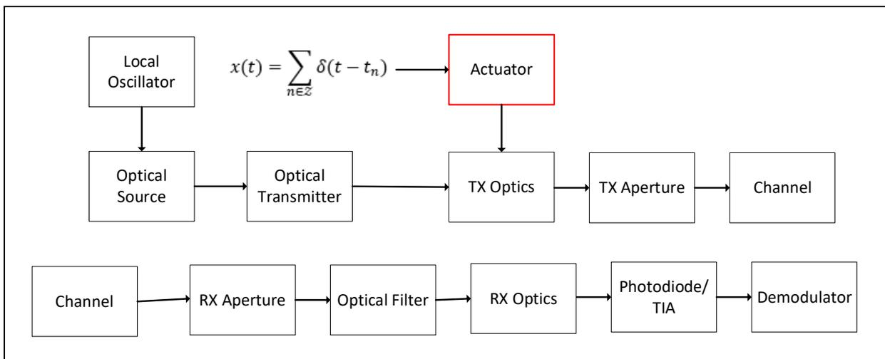
Figure 3 - Optical FRI Communications System Block Diagram
