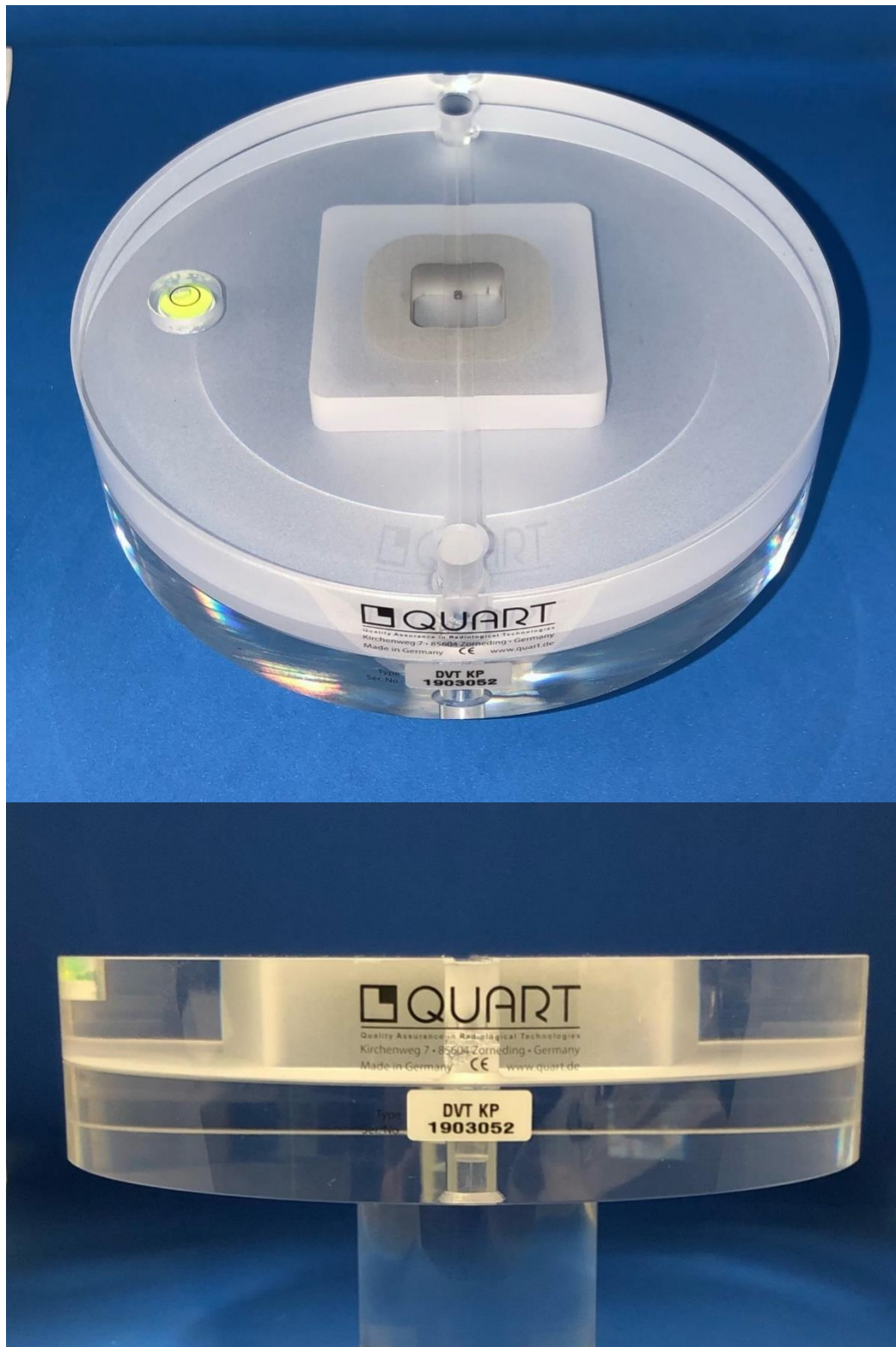
Figure 1 - Quality assurance QUART DVT phantom (QUART GmbH, Zorneding, Germany)
