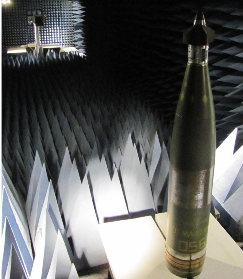
Figure 12 Anechoic chamber and M483A1 used for radiation pattern testing
