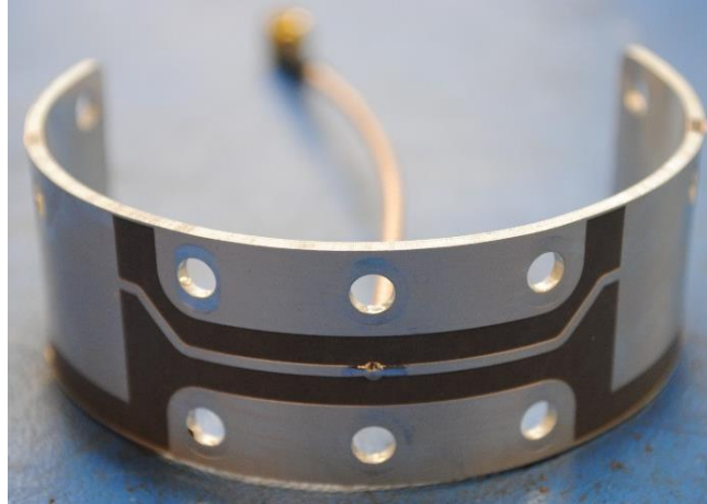
Figure 4 Fabricated wraparound antenna
