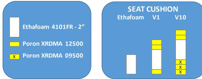
**Figure 1. Seat cushions utilized in the whole-body experiments**
