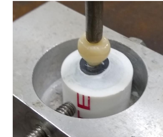
Figure: Hybrid abutment/crown in a material testing device with cylindrical piston resting in the central fossa ready for loading.
