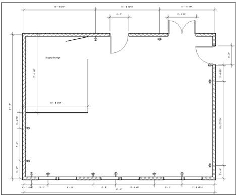
Figure C-3. Makerspace with doors, receptacles and dimensions.
