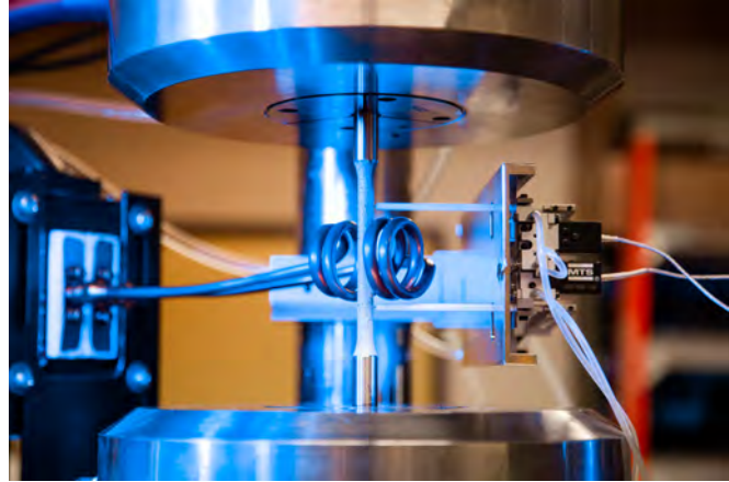
Figure 5: PI’s thermostructural rig.
