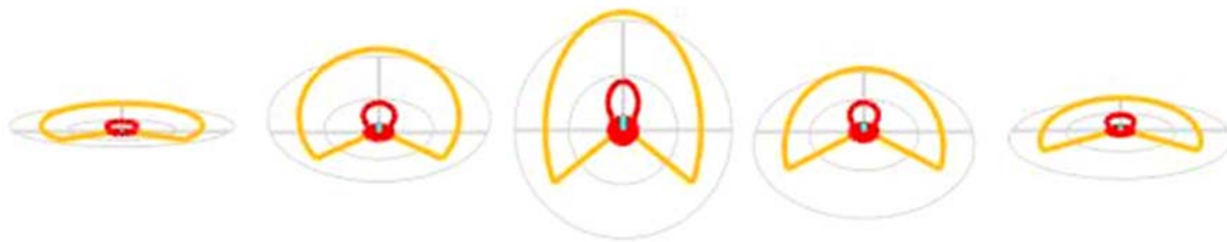
Figure 7. The 2.5D depiction of a 15-knot 3D Threat Space between +80^\circ (left) and -80^\circ (right) velocity vector elevation relative to the horizontal plane. The rotation about the lateral axis provides the 2.5D effect.
