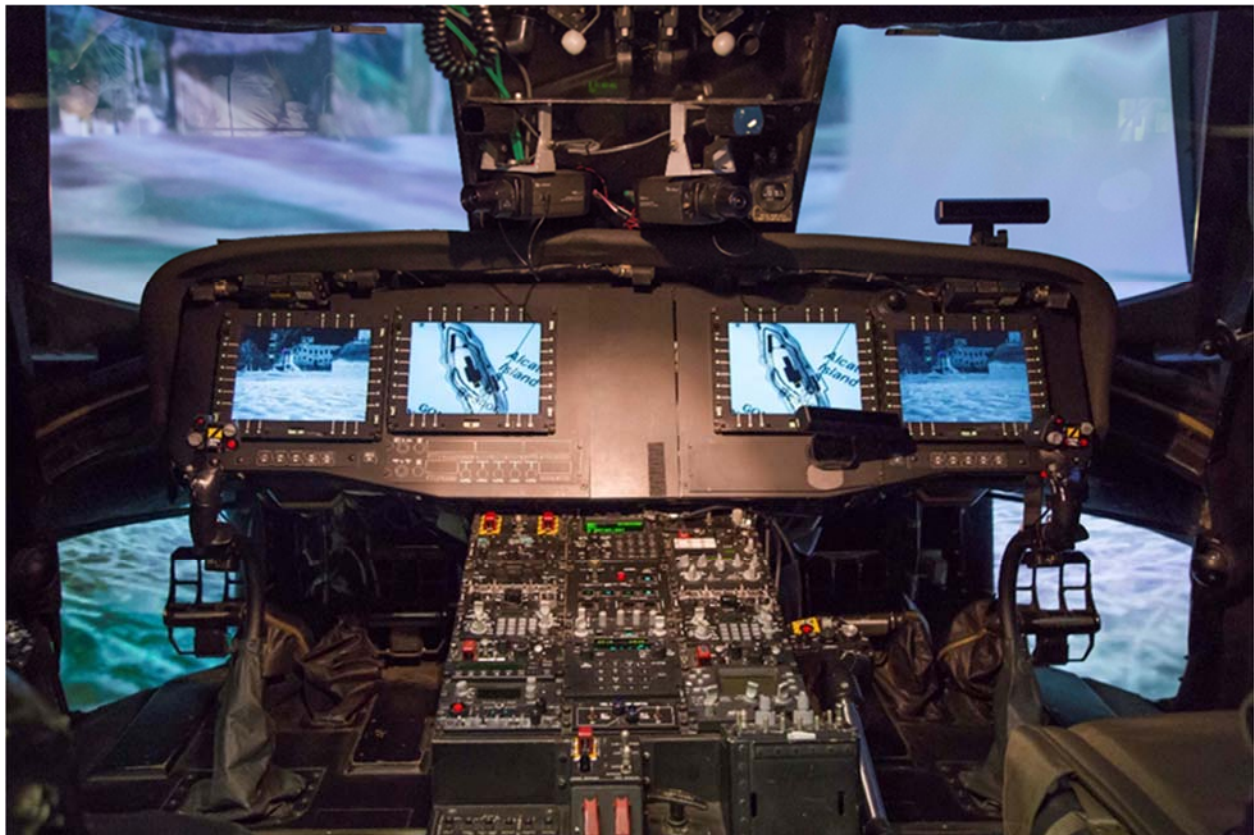
Figure 54. Cockpit with Eye Tracking Cameras in Place.
