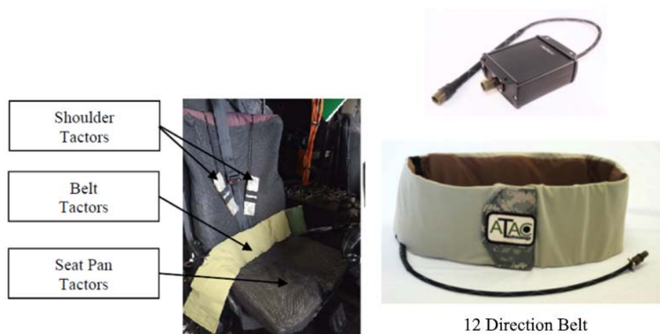
Figure 13. The Tactile Situational Awareness System (TSAS). The belt provides obstacle cueing from 12 directions, 0° forward to 330° in 30° increments.
