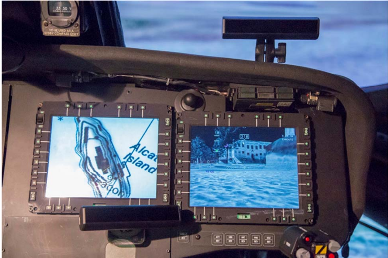
Figure 55. Cockpit with Cameras for HMD and PMD use.
