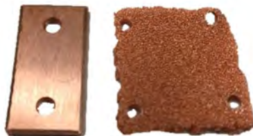
Figure 26: Solid copper (left) and copper foam (right). Holes are created for mounting to sample holder.
