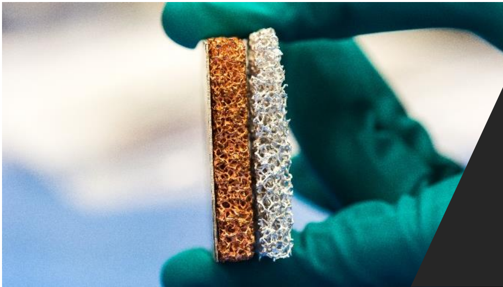
Figure 52: Dual Al-Cu foam sample.
