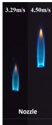
Fig. 26 Direct photographs of lifted flame with fuel jet velocities at 3.29 m/s and 4.5 m/s without ozone addition
