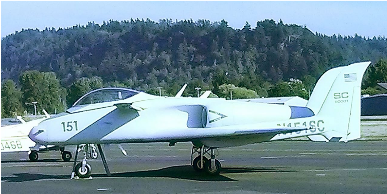
Figure 1. The Scaled Composites 151 ARES on the ramp at the Troutdale Airport (KTTD) near Portland, Oregon. View is of the left side of the aircraft, showing the engine intake. The cockpit canopy is closed. CC BY-SA 3.0, https://en.wikipedia.org/wiki/Scaled_Composites_ARES#/media/File:Scaled_Composites_ARES_151.jpg
