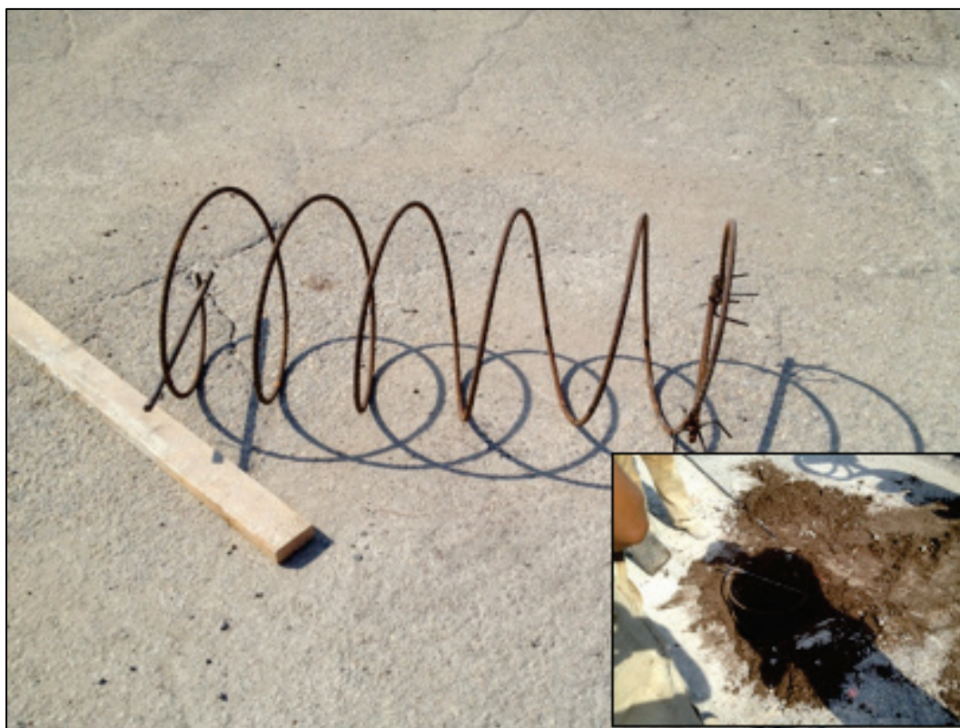
Figure 40. Spiral bent reinforcement.
