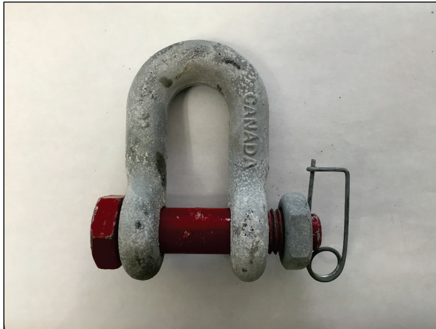
Figure 24. Shackle with quick-connecting pin installed.
