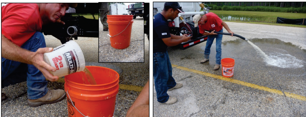
Figure B-10. Calibrating the water discharged from a water truck.
