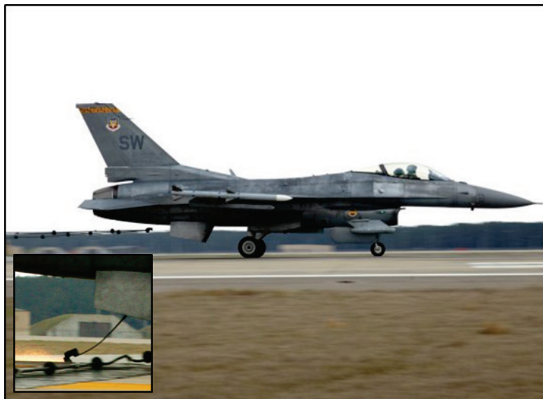
Figure 1. Operation of a pendant-based AAS (Aerospaceweb.org 2020).
