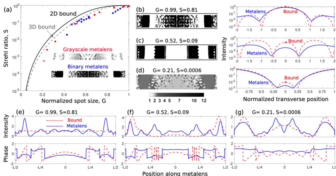
Figure 3. Inverse-designed structures that approach our superresolution bounds, across a large range of spot sizes. (e-g) show the intensity and phase of the fields at the exit planes of the metalenses, alongside the optimal profiles predicted via the bounds.
