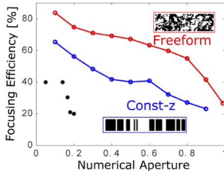
Figure 4. Our designs (const-z and freeform, corresponding to the degrees of freedom in each case) compared with previous literature (black markers).
