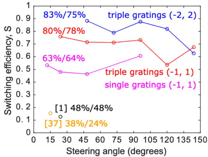
Figure 6. Comparison of our inverse-designed switchable metasurfaces (single and triple gratings) to the state-of-the-art (markers).
