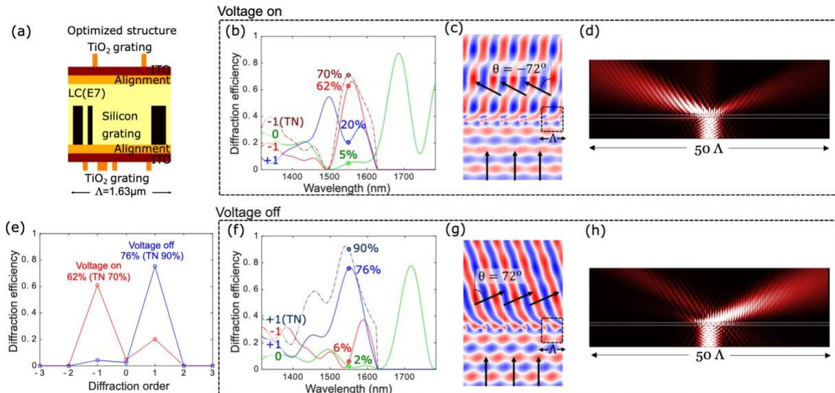
Figure 7. (a) Optimal liquid-crystal structure for 144-degree switching. (b-d) voltage-on characteristics. (f-h) voltage-off characteristics.
