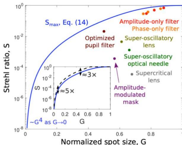
Figure 2. Comparison of global upper bound to Strehl ratio (Eq. 14) to state-of-the-art designs (colored markers). Inset: comparison of our bound (blue line) to the computational bound of Sales & Morris (back dashed), which is 3-5X larger despite applying to a much smaller set of structures (rotationally-symmetric weak scatterers).
