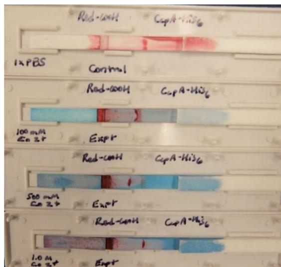
**Fig. 12** Prevention of nonspecific binding of unmodified native latex beads to CcpA-His<sub>6</sub> using cobalt(II) chloride as a divalent cation inhibitor at (top to bottom) 100, 500, and 1.0 M
