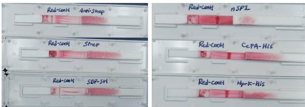
**Fig. 9** Evaluation of nonspecific binding by native, unmodified carboxylate beads. Native beads appear to have affinity for His-tagged constructs (right).
