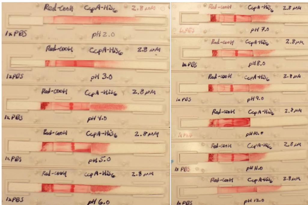
**Fig. 10** Evaluation of nonspecific binding of native red carboxylate beads to a His-tagged construct from (left) pH 2 through pH 6, and (right) pH 7 through pH 12
