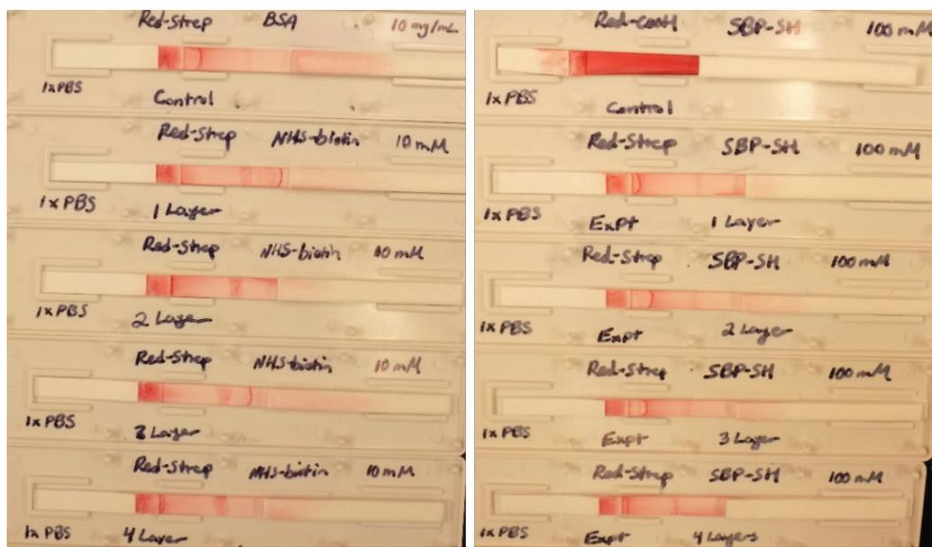
Fig. 7 Layering of (left) NHS-biotin and (right) HS-SBP. A control is included in the first row (BSA at the test line for NHS-biotin and red-COOH unfunctionalized beads for HS-SBP). Stock concentrations were 10 and 100 mM for NHS-biotin and HS-SBP, respectively. Layering is shown from one to four layers (top to bottom).
