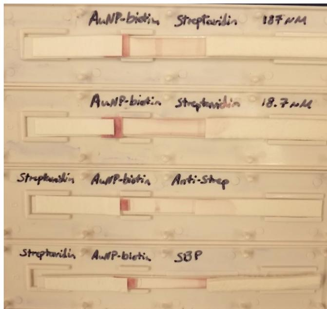
**Fig. 15** Capture of AuNP-S-PEG-biotin MW5000 reporter using (top to bottom) streptavidin at 187  $\mu$ M, streptavidin at 18.7  $\mu$ M, sandwich assay detecting 1- $\mu$ M streptavidin using anti-streptavidin as a capture agent, and sandwich assay detecting 1- $\mu$ M streptavidin using SBP as a capture agent
