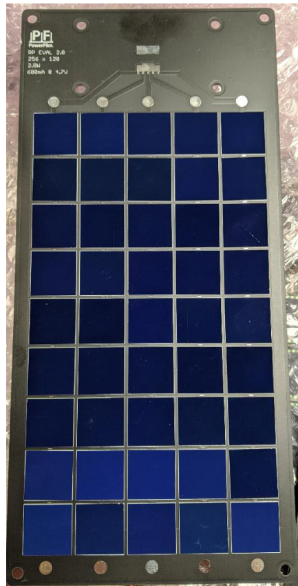
Fig. 21 SMT assembled solar array with 45 cells.
