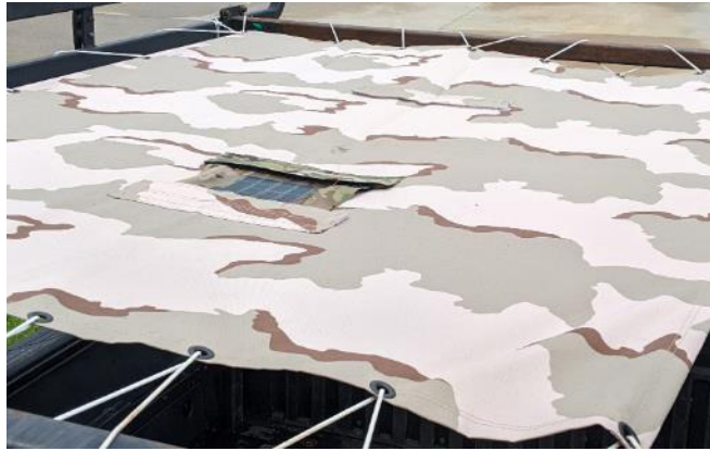
Fig. 29 Flutter test sample #4 loaded in the test fixture.
