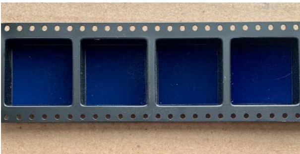
Fig. 23 Solar Cells in Tape and Reel.
